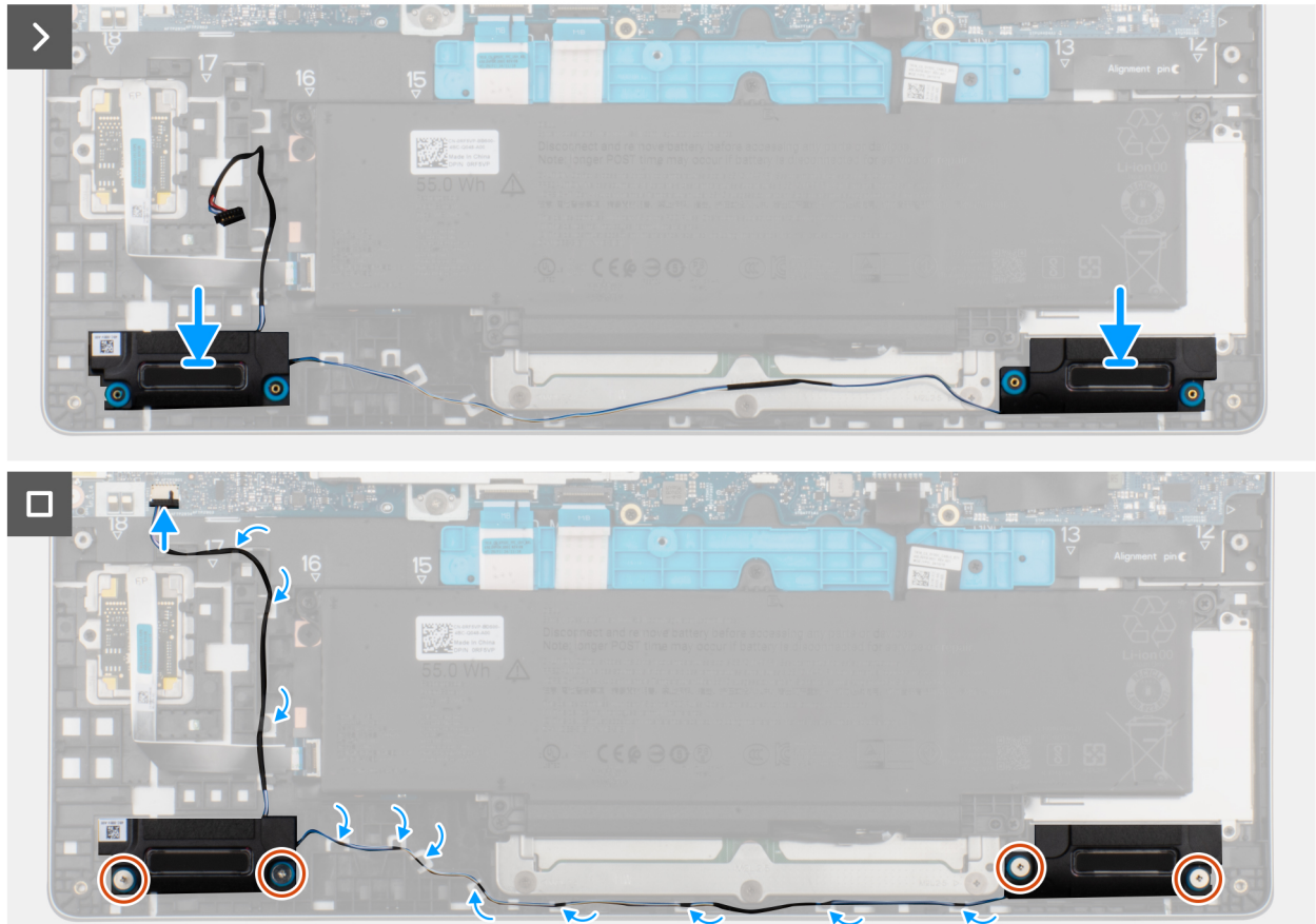
Figure 37. Installing the speakers
