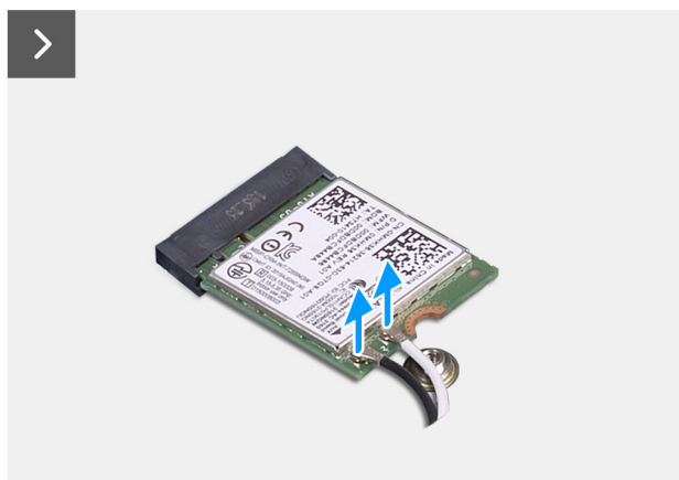
Figure 33. Removing the WLAN card
