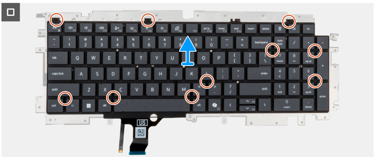
Figure 82. Removing the keyboard
