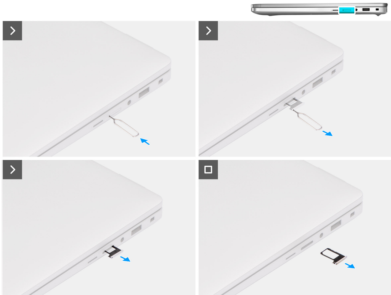
Figure 11. Removing the SIM-card tray
