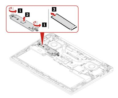
Step 2. Install the M.2 solid-state drive and M.2 solid-state drive bracket in reverse order.
