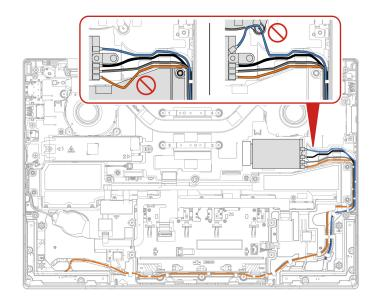
• Do not remove the plastic cover from new antenna connectors until you install the new antennas.
