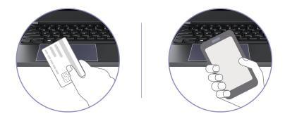
Note: Ensure that the NFC card is in NFC Data Exchange Format (NDEF), otherwise the card cannot be detected.
