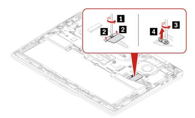
Step 2. Install the captive bracket and wireless WAN module bracket in reverse order.
