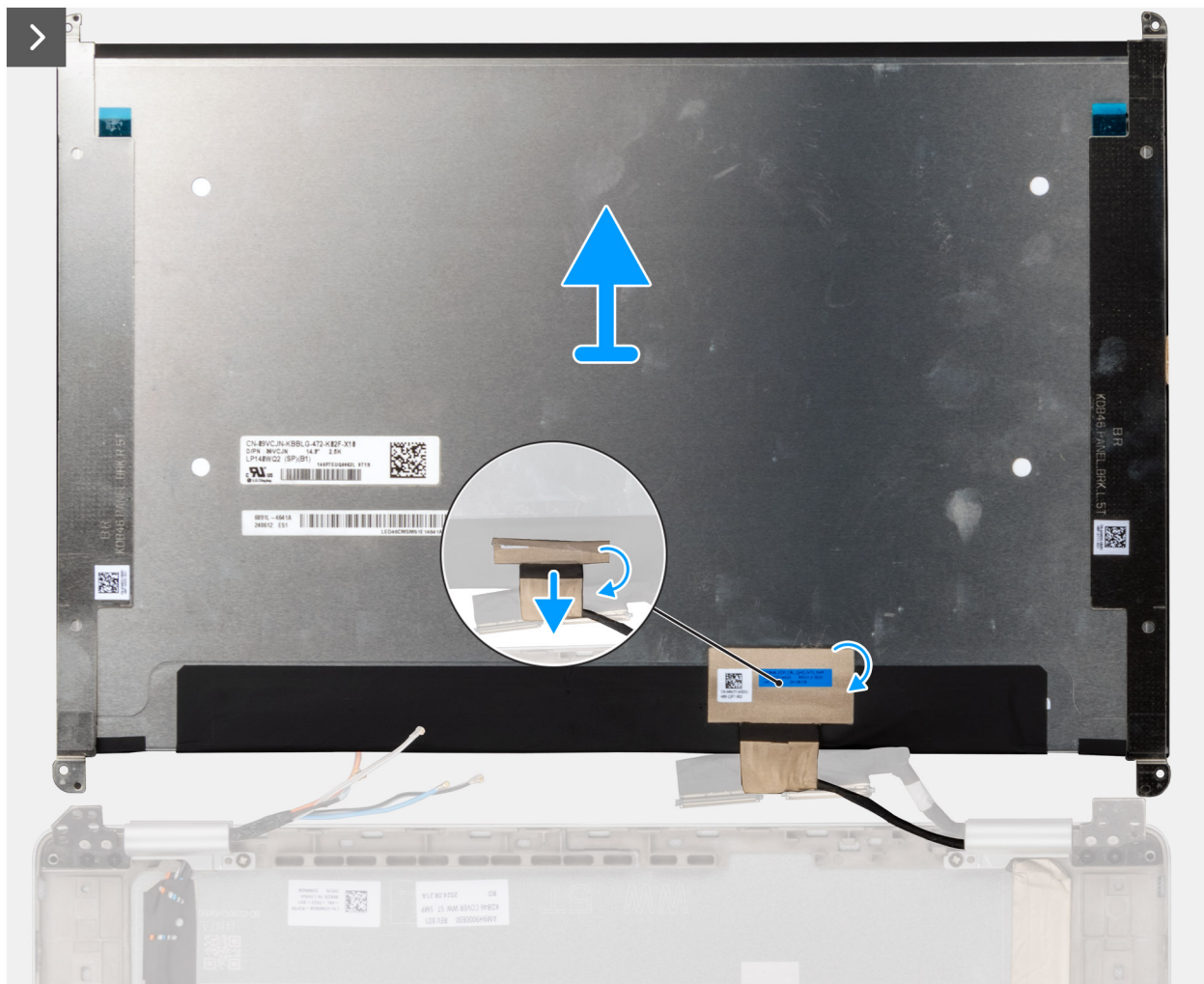
Figure 73. Removing the display panel
