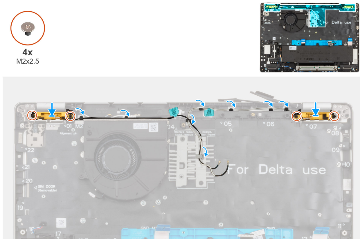
Figure 77. Installing the wireless antenna
