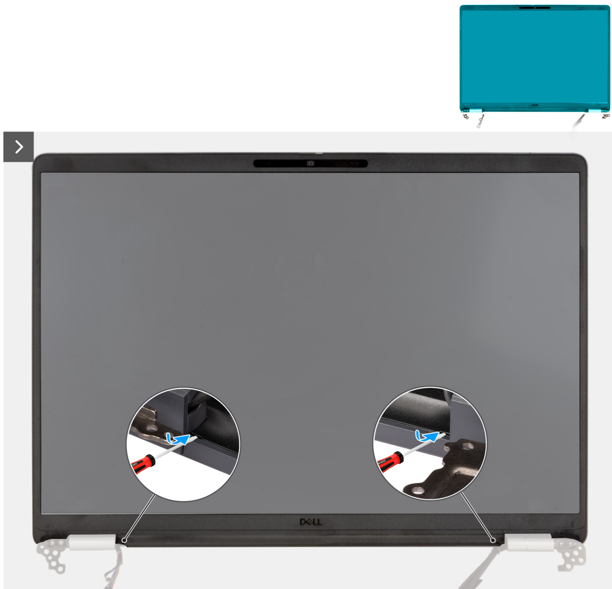
Figure 61. Prying the plastic bezel
