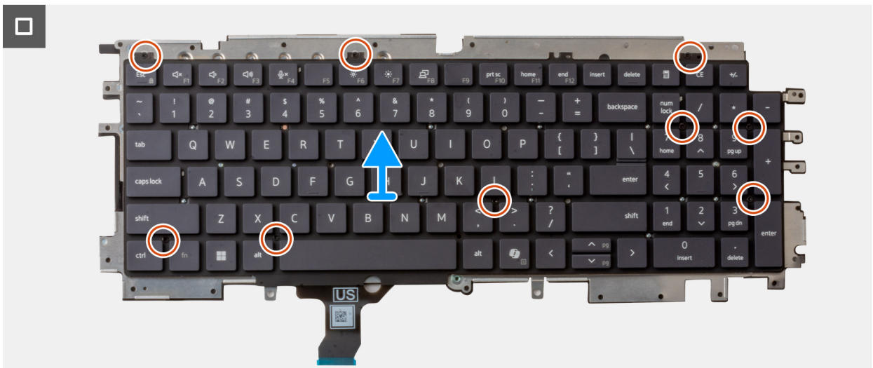
Figure 79. Removing the keyboard
