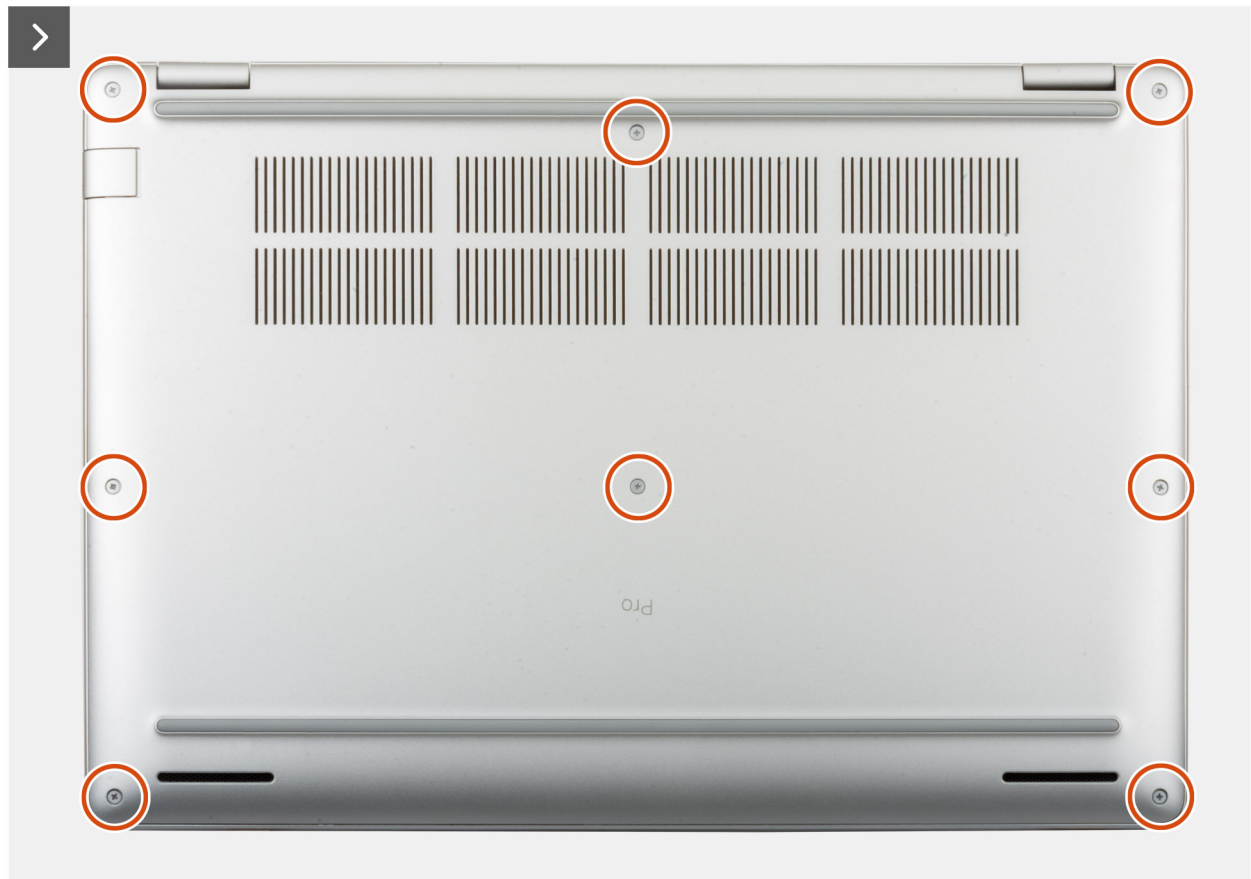
Figure 13. Removing the base cover
