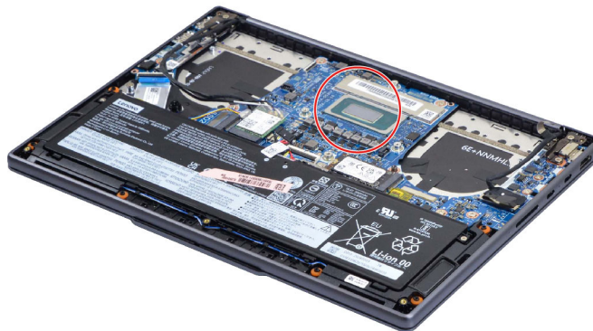
Figure 5. Areas on the system board where thermal interface materials are applied
