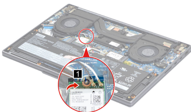
Figure 12. Remove the Wi-Fi card mylar
