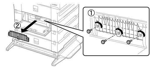
6. Slide out two used pickup rollers, and remove both of them.
