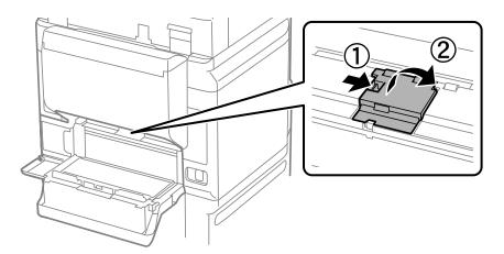
7. Slide out the two used pickup rollers, and remove them.
