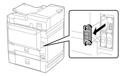
4. Install the ethernet board straight into the additional interface slot for the ethernet board.
