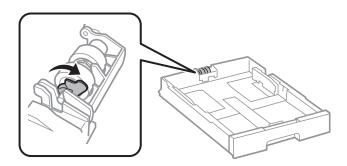
11. Slide the pickup roller toward the lever, and then remove them by taking the shaft out of the holder.
