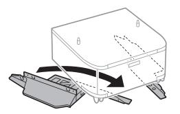
6. Secure the stands with the attachments and screws.
