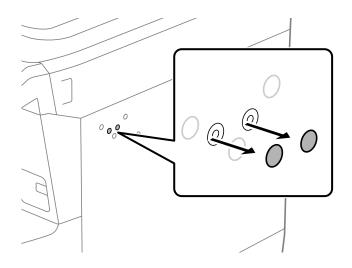
2. Using a Phillips screwdriver, secure the metal plate (g) with the two screws (e).
