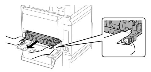
6. Remove the cover inside the back of the printer.
