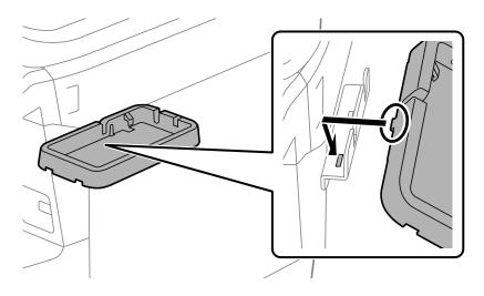
4. Secure the bottom part (b) of the authentication device stand with the screws (c). Turn the screw (c) by hand.
