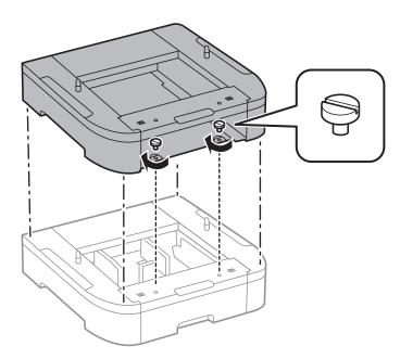
8. Lower the printer gently onto the paper cassette unit aligning the corners, and then secure them with the screws.
