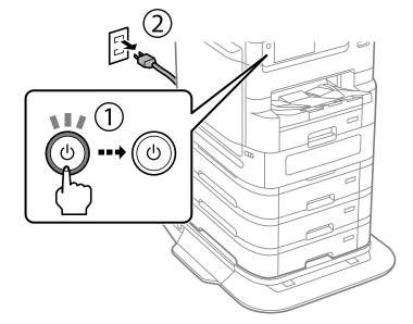
1. Turn off the printer by pressing the 0 button, and then unplug the power cord.
