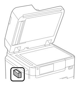
3. Use the cleaning cloth to clean the surface of the scanner glass.
