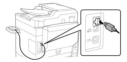
10. Remove the seal, attach the clamp, and then connect the cable, as shown below.
