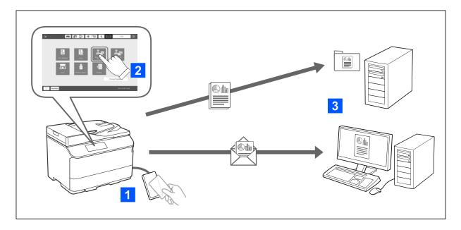
You can use the printer's control panel functions (scanning, copying, faxing, etc.) by logging in to the printer as an authenticated user.
