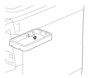
5. Place the upper part (a) on to the authentication device stand as shown in the illustration.
