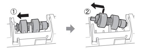
12. Insert the shaft of the new pickup roller into the hole in the holder, and then slide the shaft on the lever side along the slot while it is facing the flat surface at the front.
