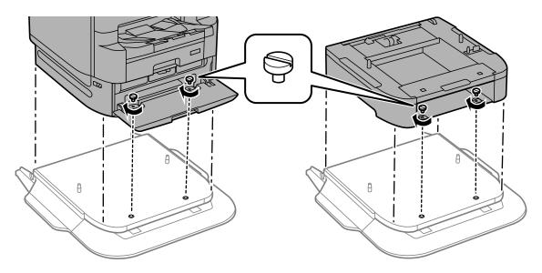
If the printer stand is attached to the paper cassette unit, lower the printer gently onto the paper cassette unit aligning the corners, and then secure them with the screws.
