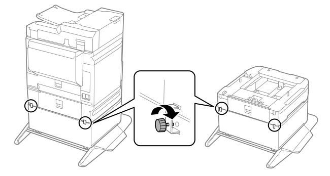
12. Secure the printer or an optional paper cassette unit at the back with the attachments and screws.
