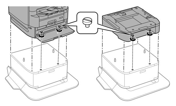
If the cabinet is attached to the paper cassette unit, lower the printer gently onto the paper casette unit aligning the corners, and then secure them with the screws.
