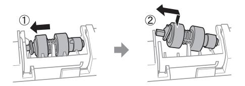
14. Insert the shaft of the new pickup roller into the hole in the holder, and then slide the shaft on the lever side along the slot while it is facing the flat surface at the front.
