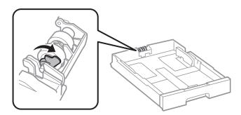
13. Slide the pickup roller toward the lever, and then remove them by taking the shaft out of the holder.
