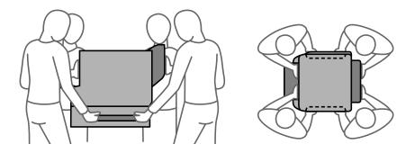
U When carrying the printer, do not tilt it more than 10 degrees; otherwise the printer may fall.
