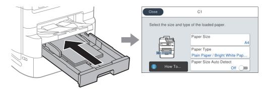
If displayed paper size and type differ from the loaded paper, select the item to change. If the settings match the loaded paper, close the screen.
