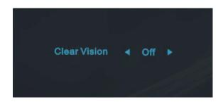
3. Press and hold the "<" button for 5 seconds to activate the Clear Vision demo, and the message "Clear Vision Demo: on" will appear on the screen. Press the menu or exit button, and the message will disappear. Press and hold the ' <' button again for 5 seconds to close the Clear Vision demonstration.(Clear Vision demo: On) Five seconds.
