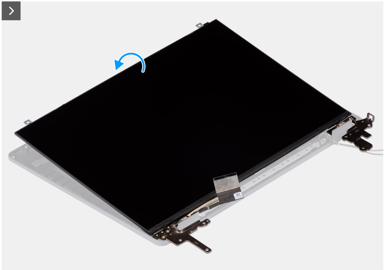
Figure 80. Installing the display-panel assembly
