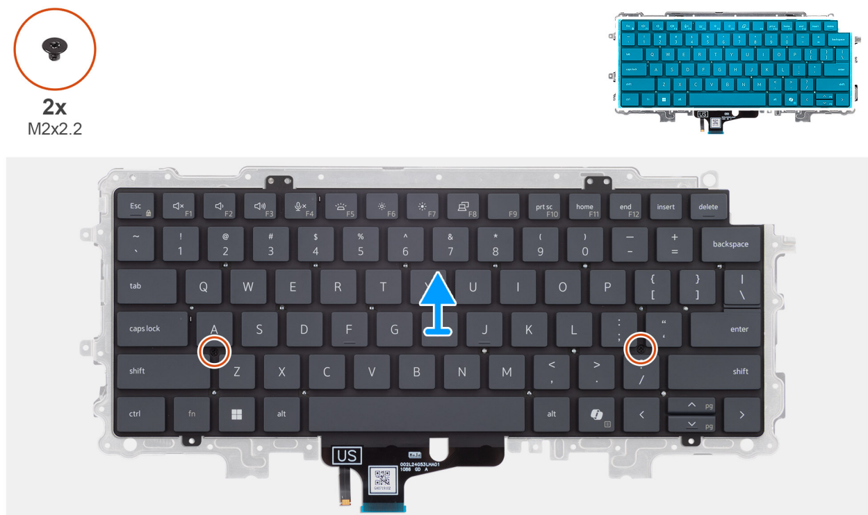
Figure 56. Removing the keyboard support plate
