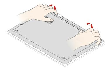
Step 2. Install the base cover assembly in reverse order.
