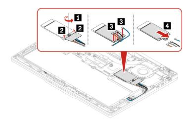
Step 2. Install the captive bracket and wireless WAN module in reverse order.
