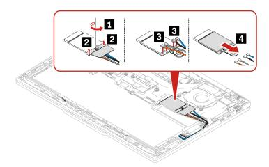
Step 2. Install the captive bracket and wireless WAN module and its bracket in reverse order.
