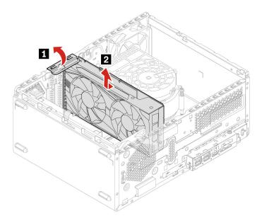
Note: If the card is held in place by the retaining latch, press the latch as shown to disengage the latch. Then, gently remove the card from the slot.
