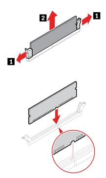
Note: During the installation, ensure that you align the memory module to the slot and press down on both ends until the latches are fully engaged with a click.
