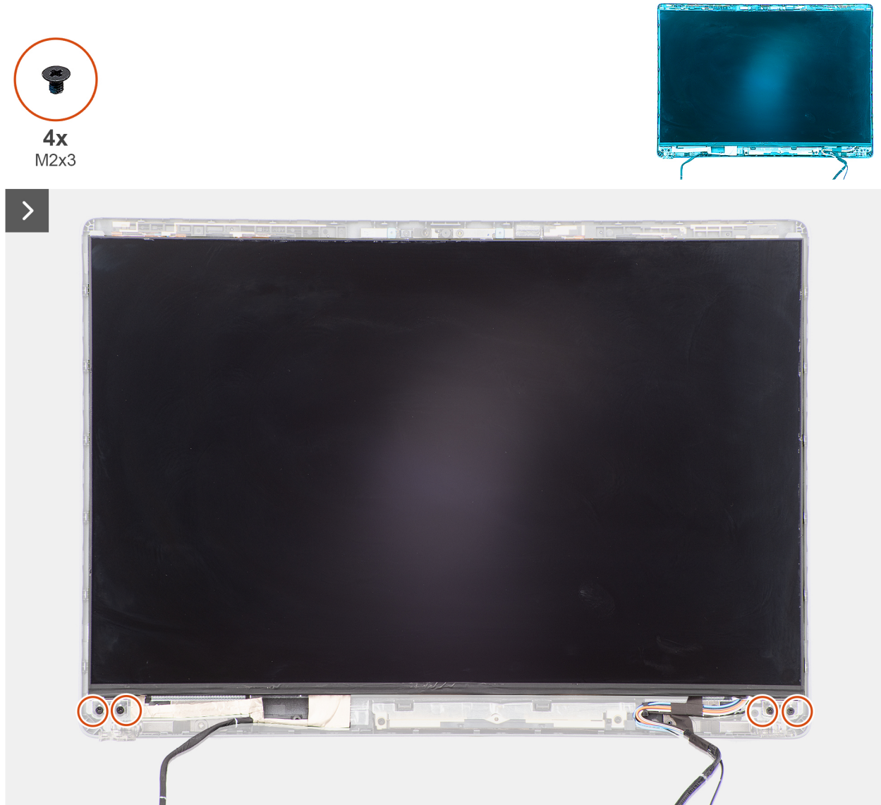
Figure 68. Removing the display panel
