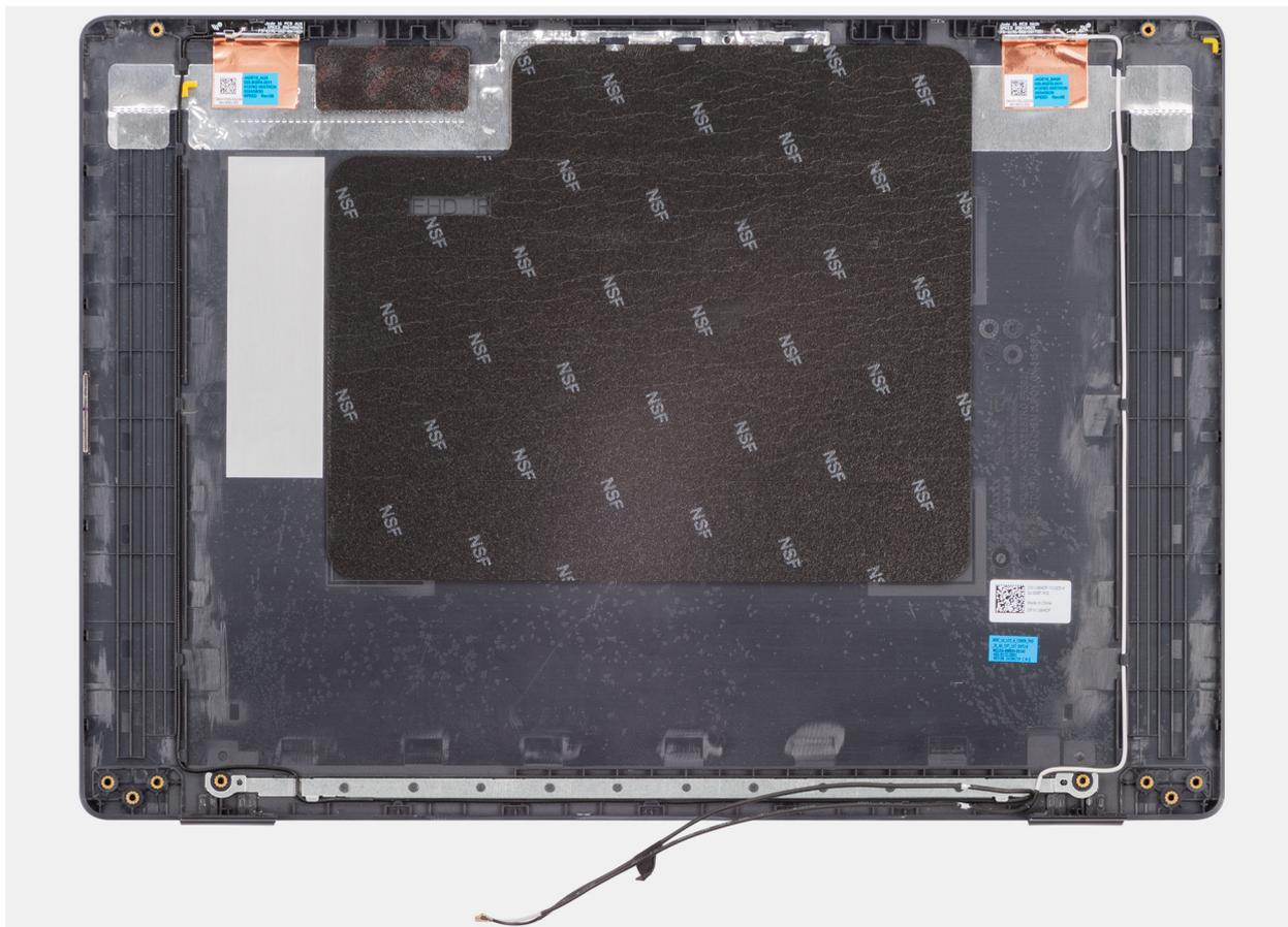
**Figura 97. Installing the display back-cover assembly**
