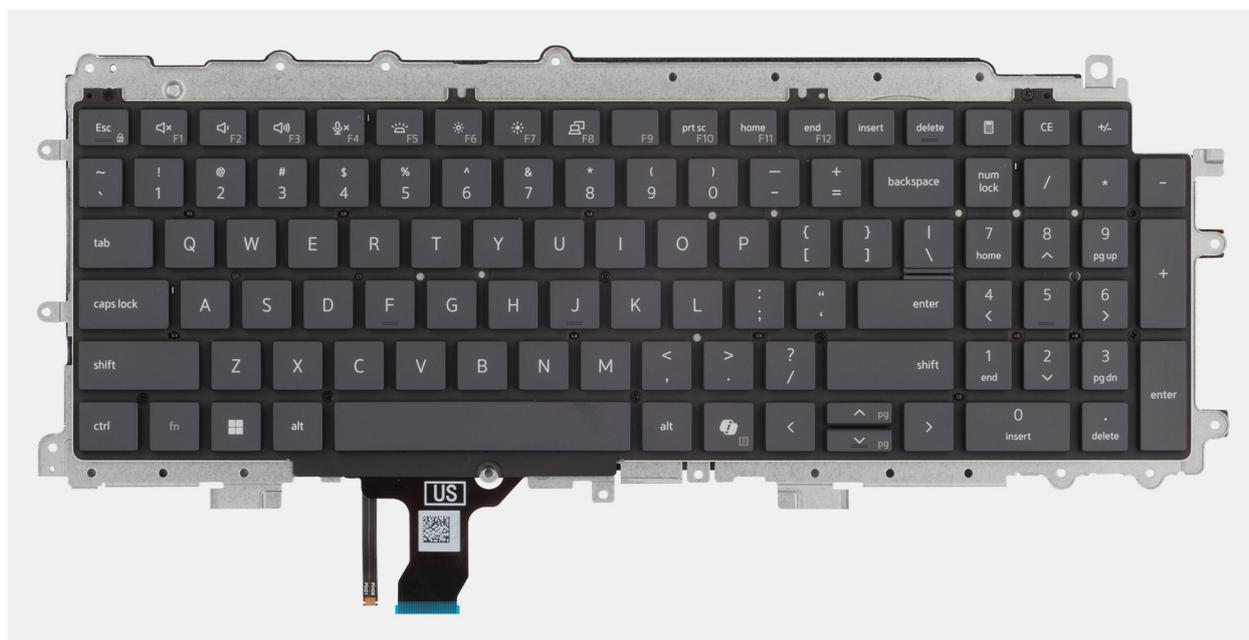
Figura 62. Removing the keyboard
