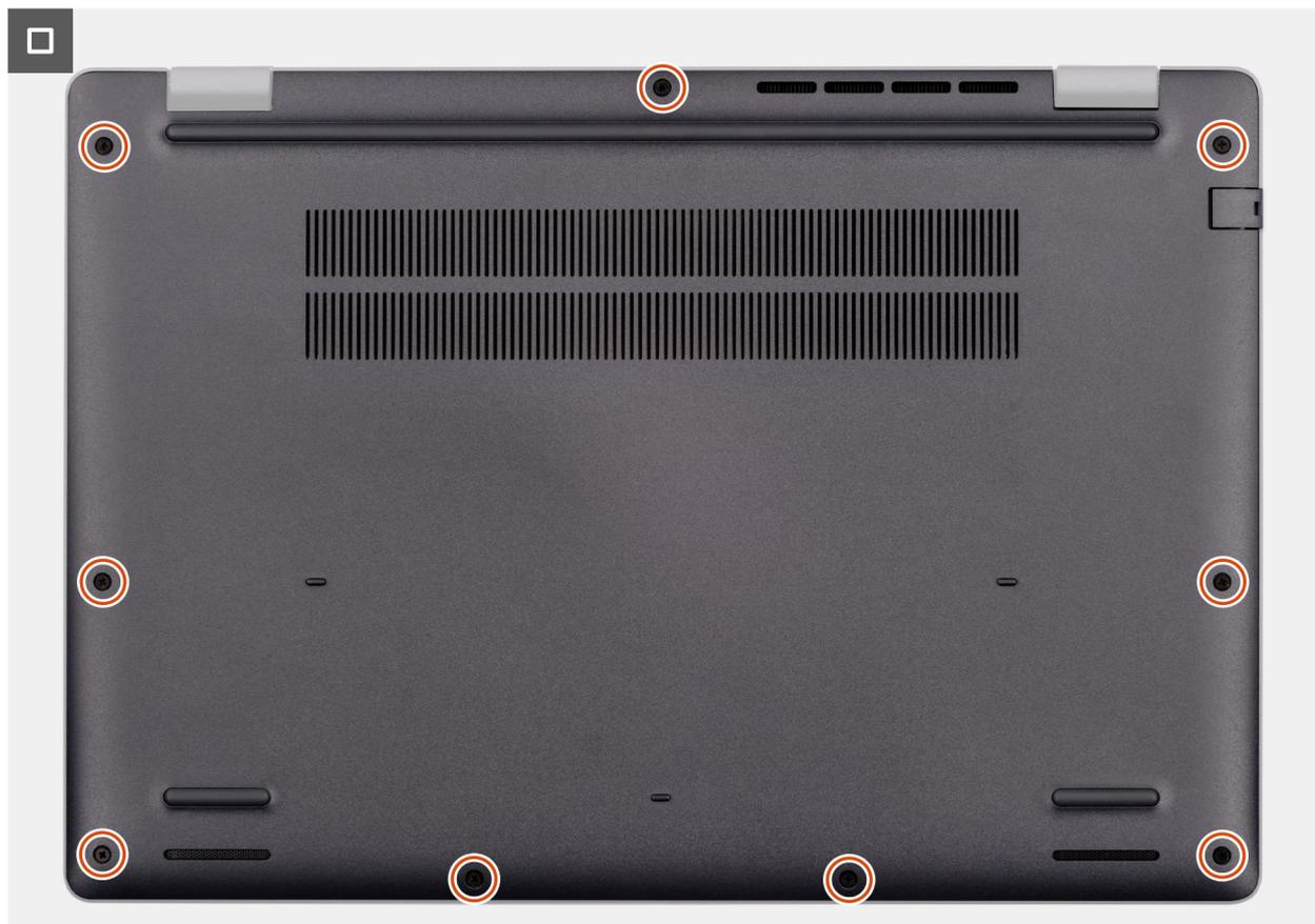
Figura 16. Installing the base cover
