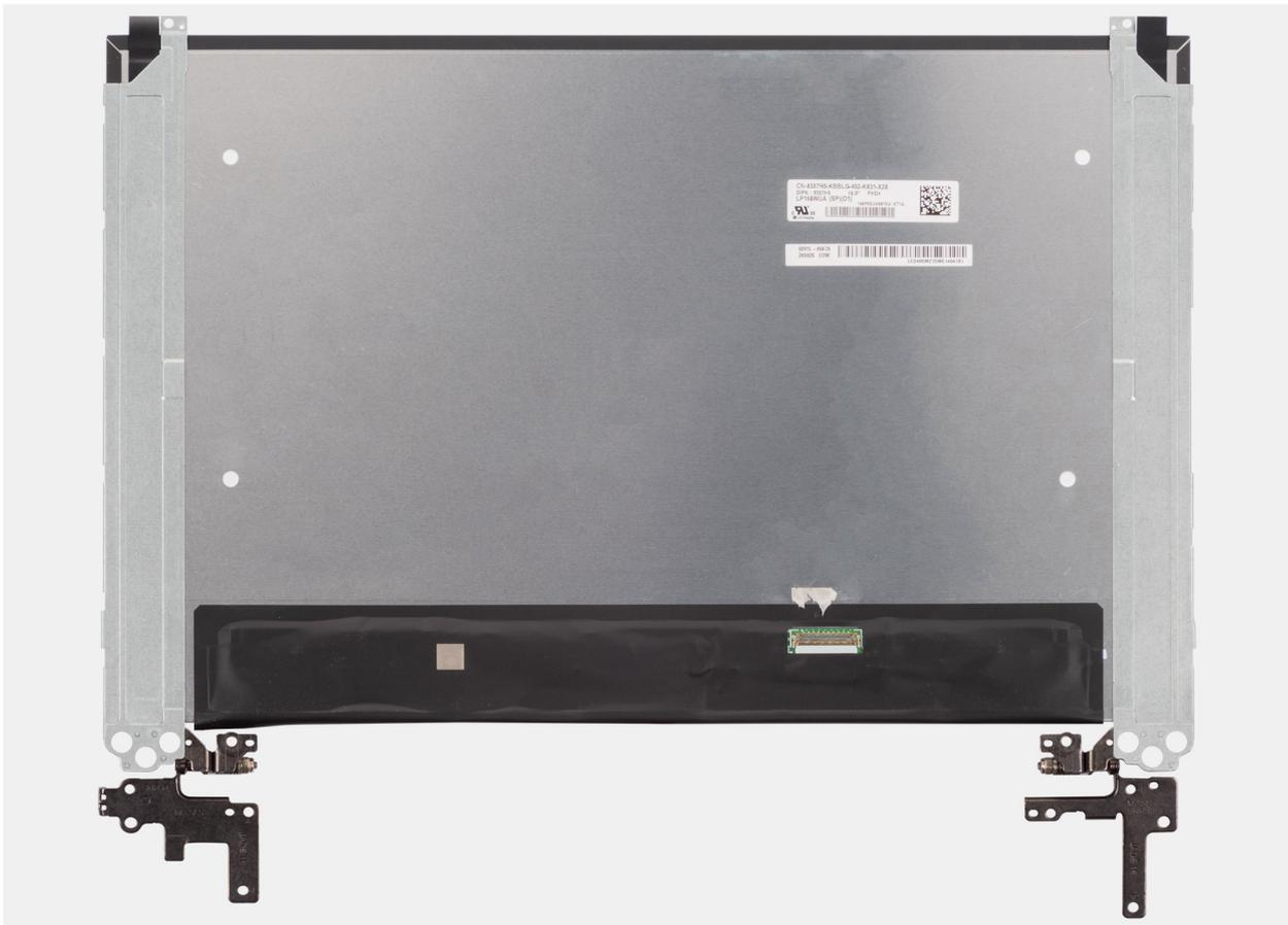
1. Remove the six (M2.5x2.5) screws and four (M2.5x3.5) screws that secure the left and right hinges to the display back cover.
