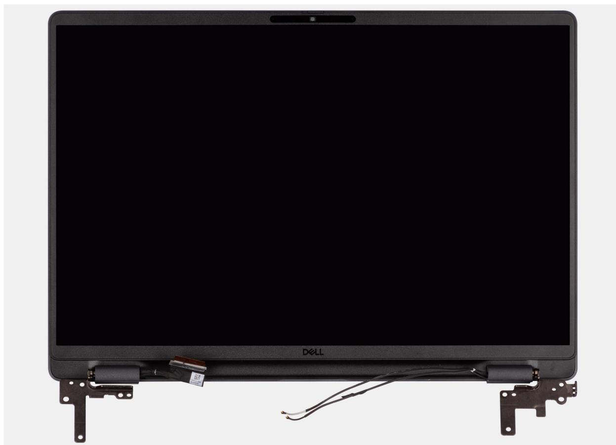
Figura 74. Removing the display assembly
