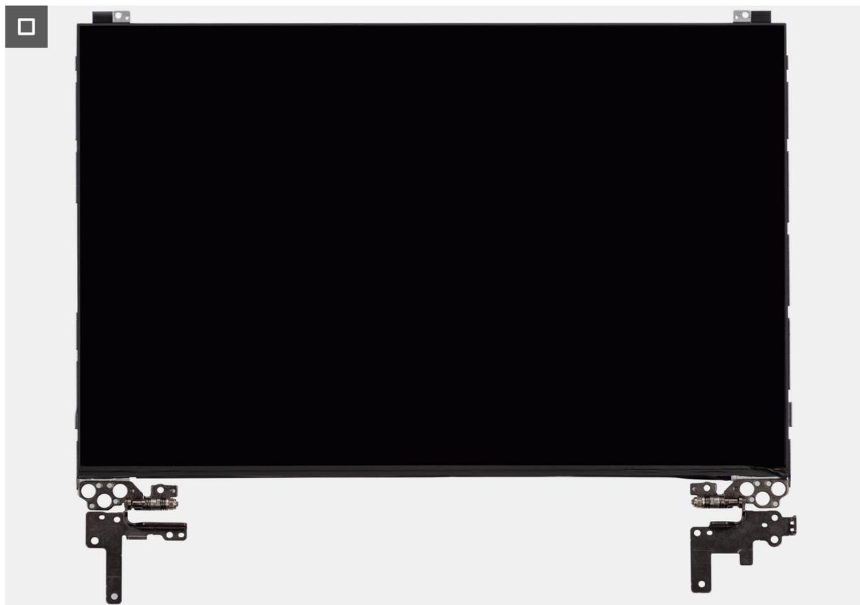
**Figura 87. Removing the display-panel assembly**
