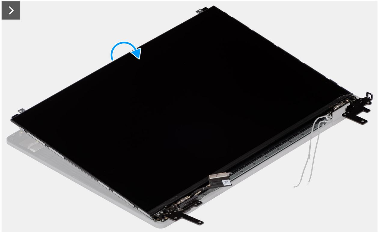
Figura 85. Removing the display-panel assembly
