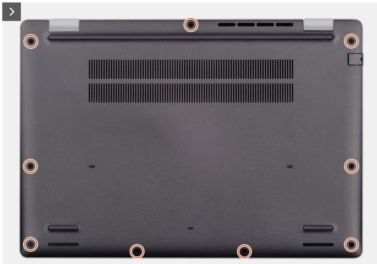
Figura 11. Removing the base cover
