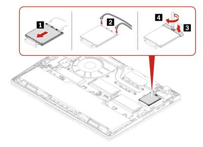
**Note:** When installing the wireless WAN module, ensure that you connect the orange cable to the connector labeled Orange on the module, and the blue cable to the connector labeled Blue.
