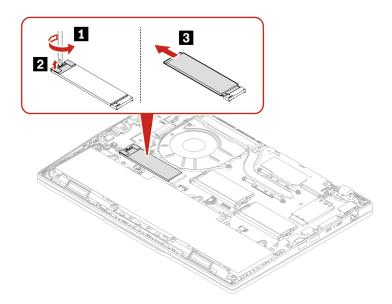
Step 2. Install the 2280 M.2 solid-state drive and its bracket in reverse order.
