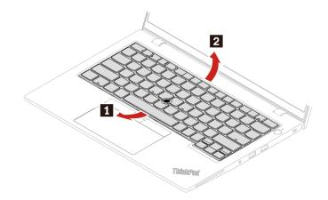
Step 4. Put the keyboard on the palm rest as shown and detach the connectors. Then, remove the keyboard.
