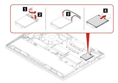
Step 2. Install the wireless WAN module and its bracket as shown below.
