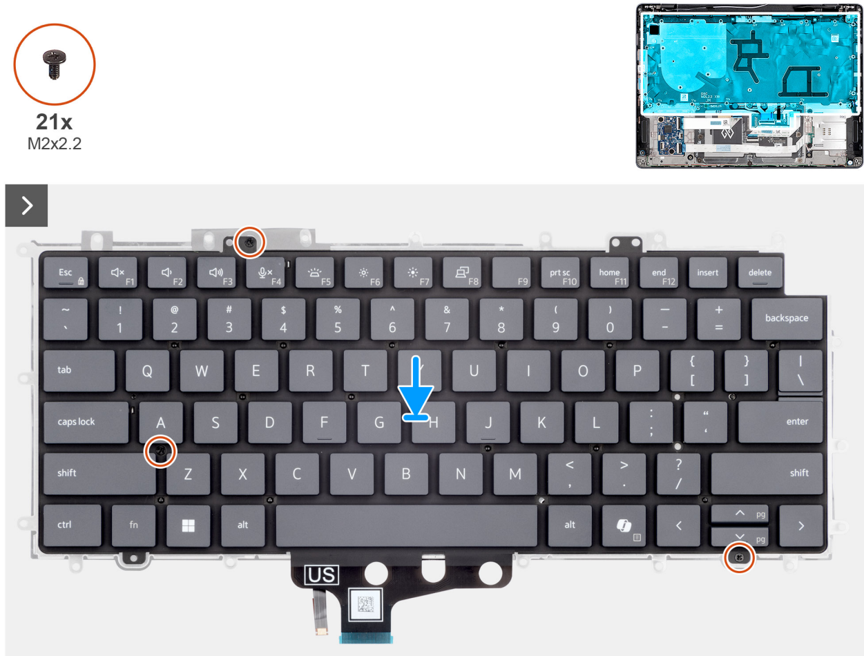
Figure 97. Installing the keyboard
