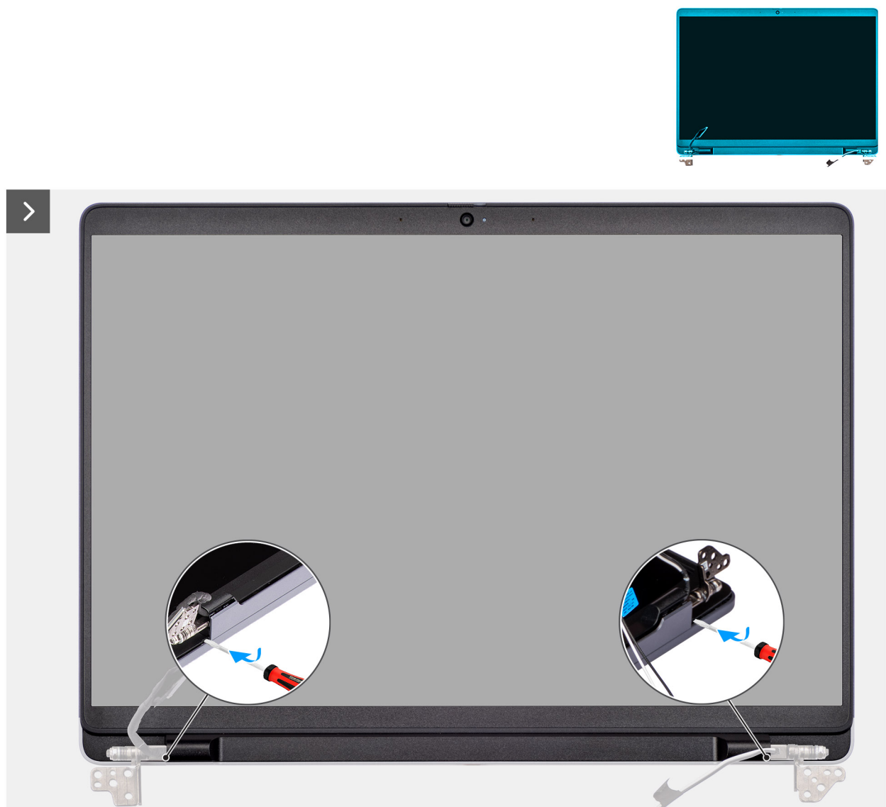
Figure 52. Removing the display bezel
