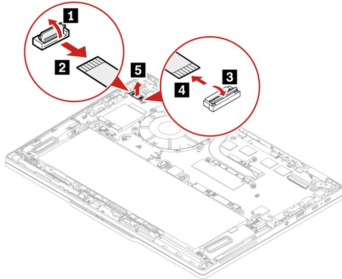
Step 3. Install the power button with fingerprint reader and fingerprint reader cable in reverse order.
