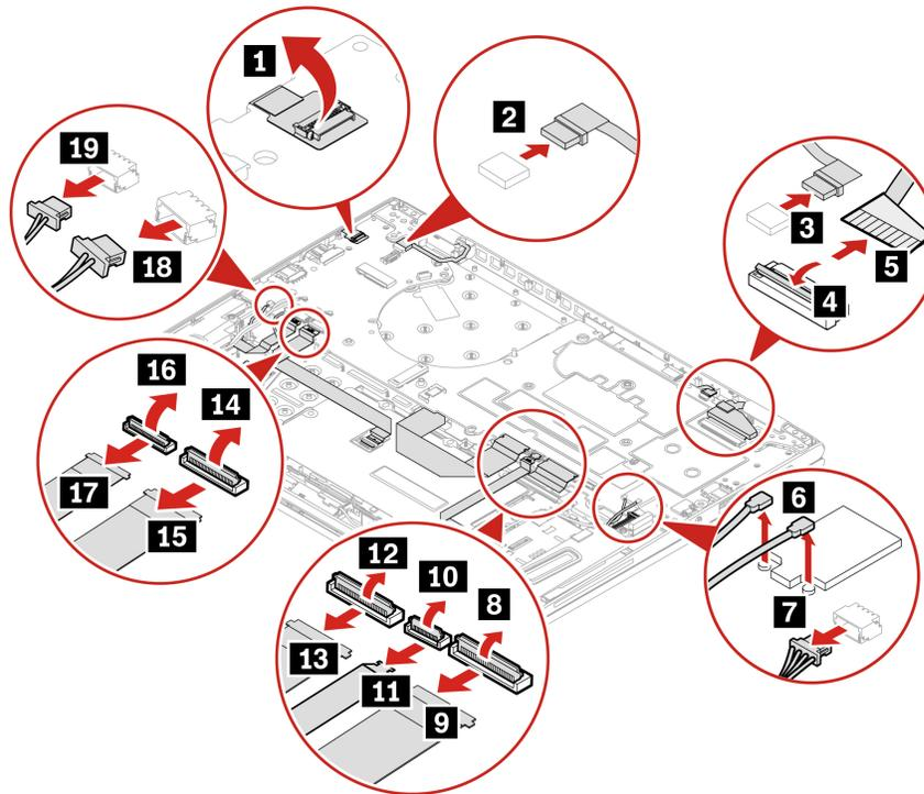
Remove the system board as shown below.
