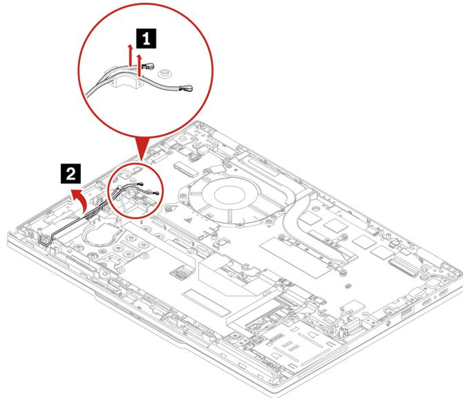
Step 2. Remove the wireless WAN antenna assembly as shown below. (When installing, ensure that the gasket **a** on copper-foil is under the trackpad bracket.)
