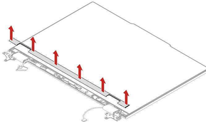
Step 2. Install the LCD stripe cover in reverse order. When installing, ensure that all the latches are attached firmly.
