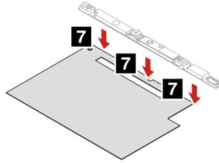
Step 2. Install the camera-and-microphone module in reverse order.
