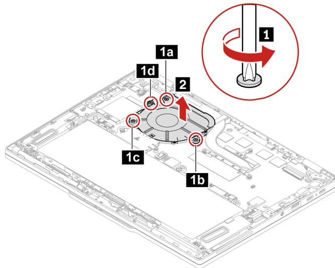
Step 2. Install the thermal fan assembly in reverse order.
