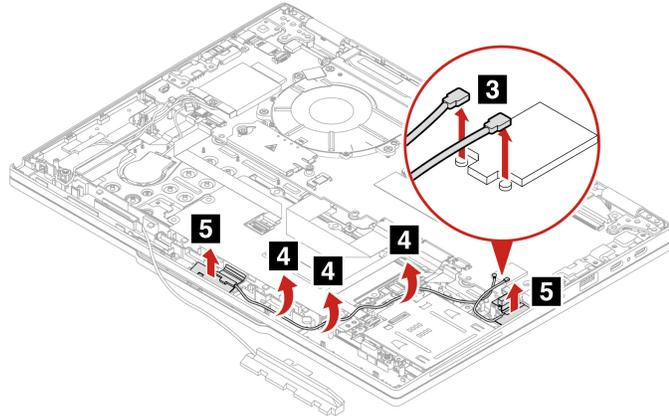
Step 3. Install the wireless WAN antenna assembly in reverse order.
