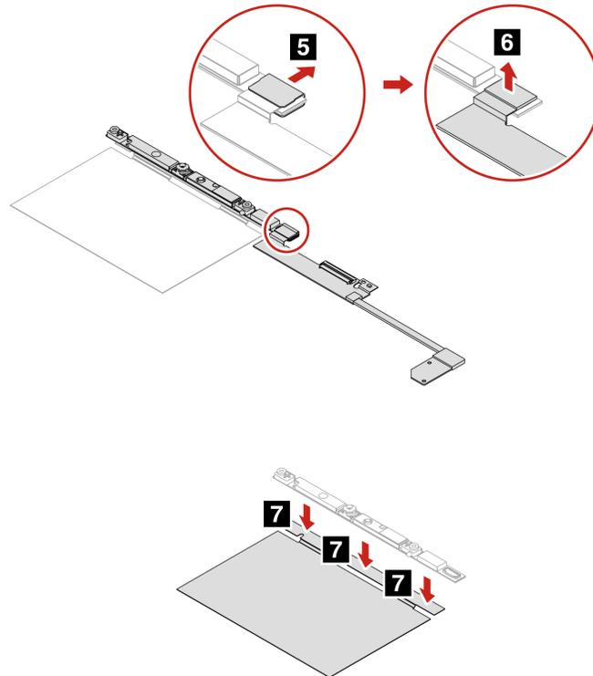
Step 2. Install the camera-and-microphone module in reverse order.
