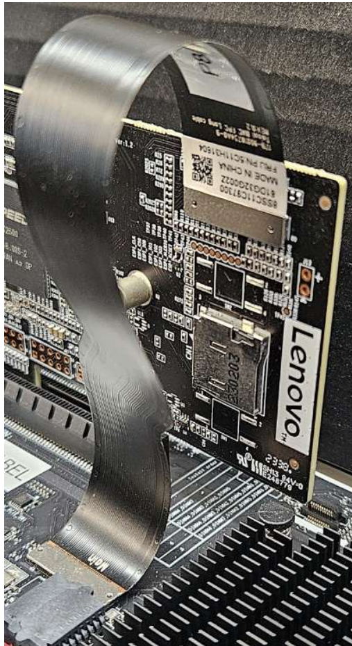
Figure 15, Sideband cable into the BMC card port in Slot 8 on the PX
