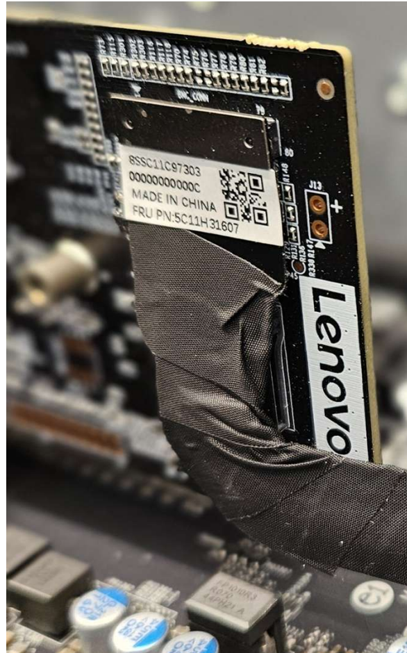
Figure 27, Sideband cable into the BMC card port in Slot 5 on the PX
