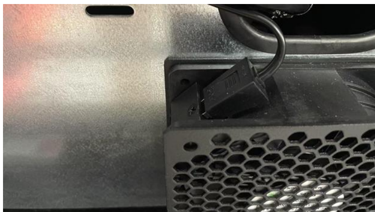
Figure 14 – Connecting the Fan Power Cable to the HyperShelf
