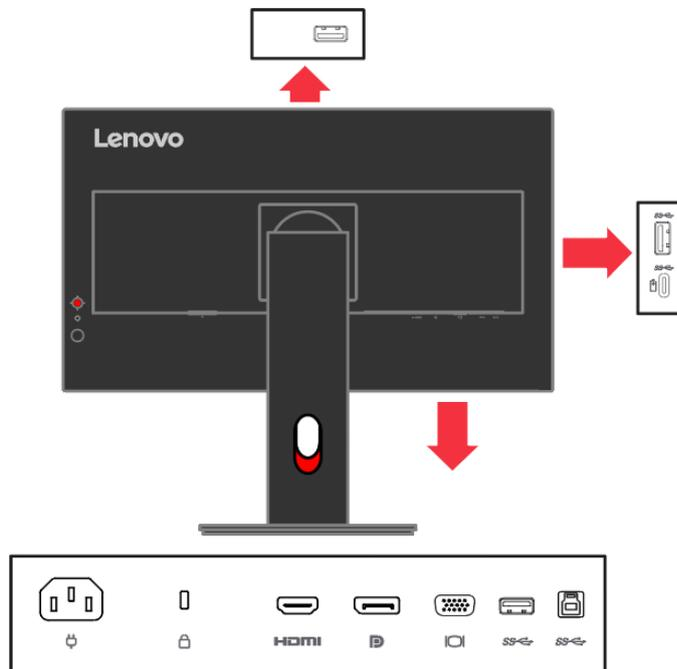
3. Connect one end of the DP cable to the DP connector on the back of the computer, and the other end to the DP connector on the monitor. Lenovo recommends that customers who require using the DisplayPort input on their monitor purchase the "Lenovo DisplayPort to DisplayPort cable 0A36537".
