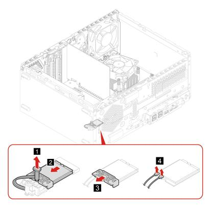
**Note:** During installation, ensure that you connect the gray cable to the connector labeled AUX on the card, and the black cable to the connector labeled MAIN.
