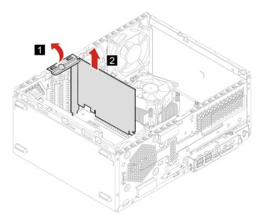
**Note:** If the card is held in place by retaining latch, press the latch as shown to disengage the latch, Then, gently remove the card from the slot.
