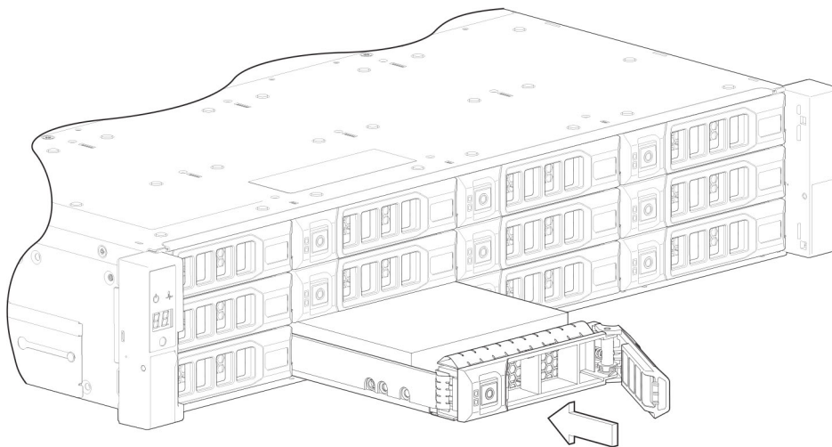
Figure 41. Installing an LFF drive carrier module (1 of 2)
