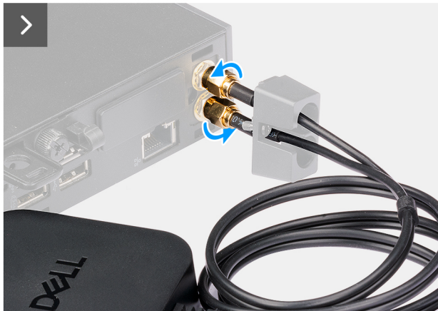
Figure 34. Removing external puck antenna
