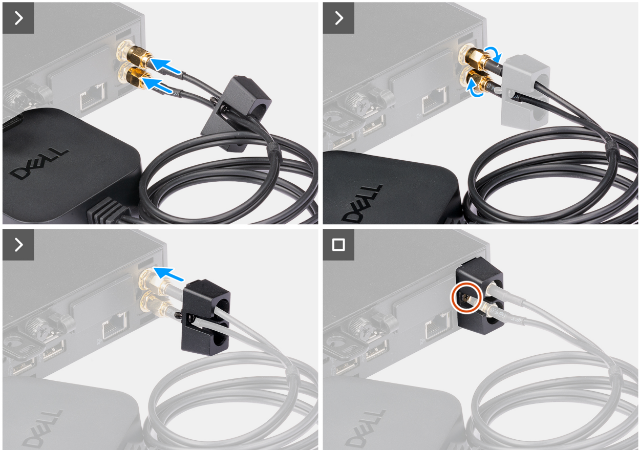
Figure 35. Installing external puck antenna
