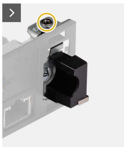
Figure 74. Installing the antenna module (white cable)
