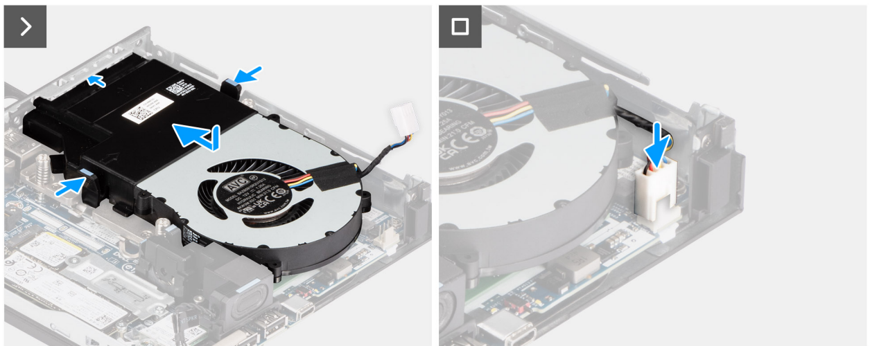
Figure 31. Installing the fan
