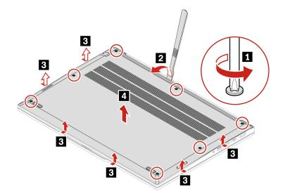
Step 2. Install the base cover assembly in reverse order.
