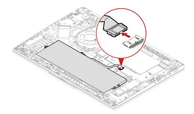
b. Loosen the three captive screws and remove the battery as shown below.
