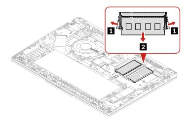
Step 2. Install the memory module as shown below.
