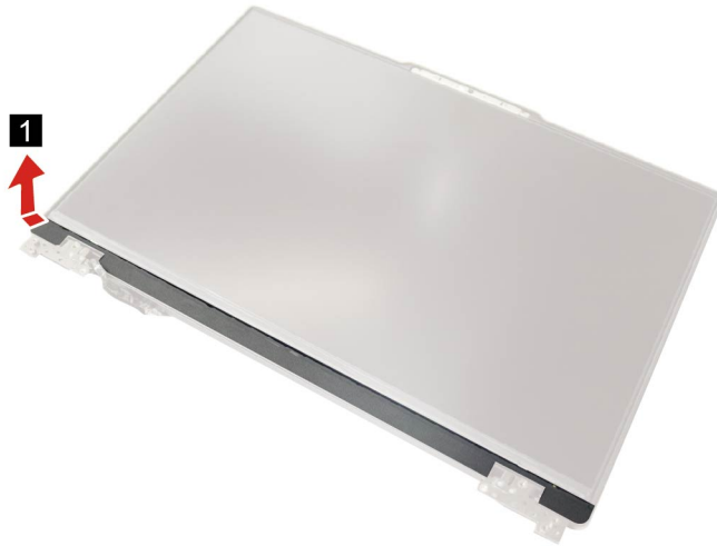
Figure 32. Remove the hinge cover
