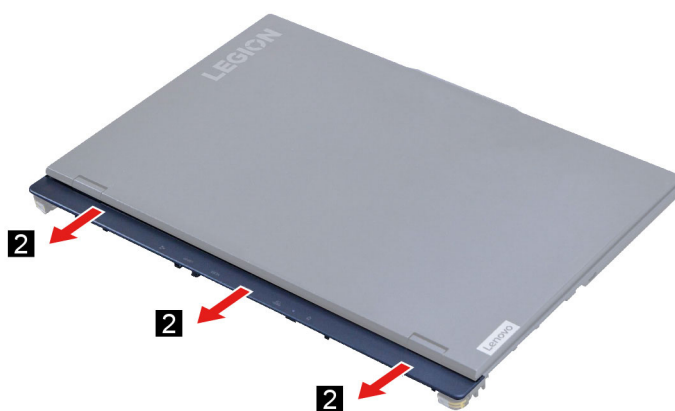
Figure 49. Remove the strip cover
