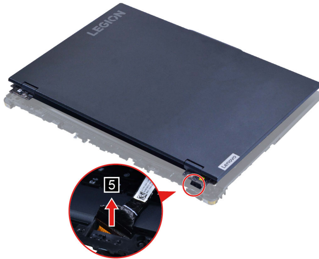
Figure 52. Take out the EDP cable and remove the LCD module
