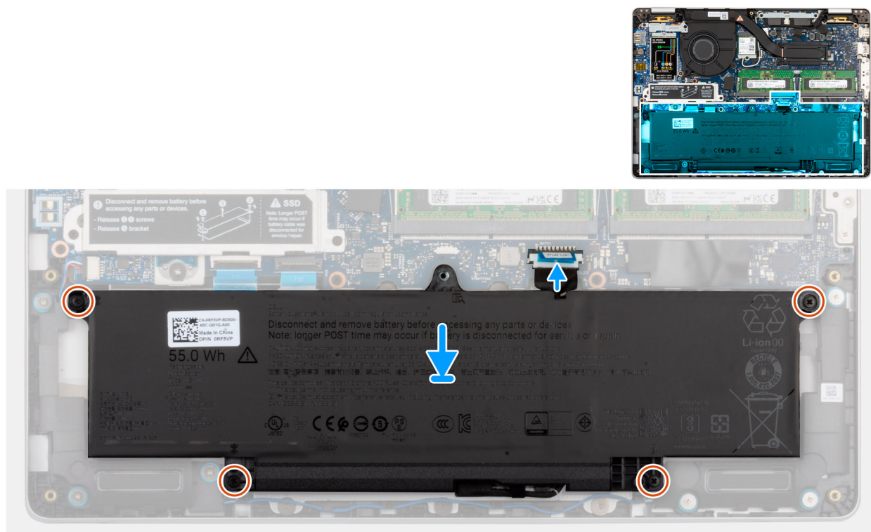
Figure 20. Connecting the battery cable
