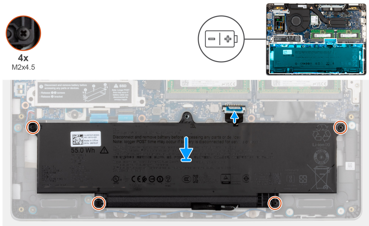
Figure 24. Installing the battery
