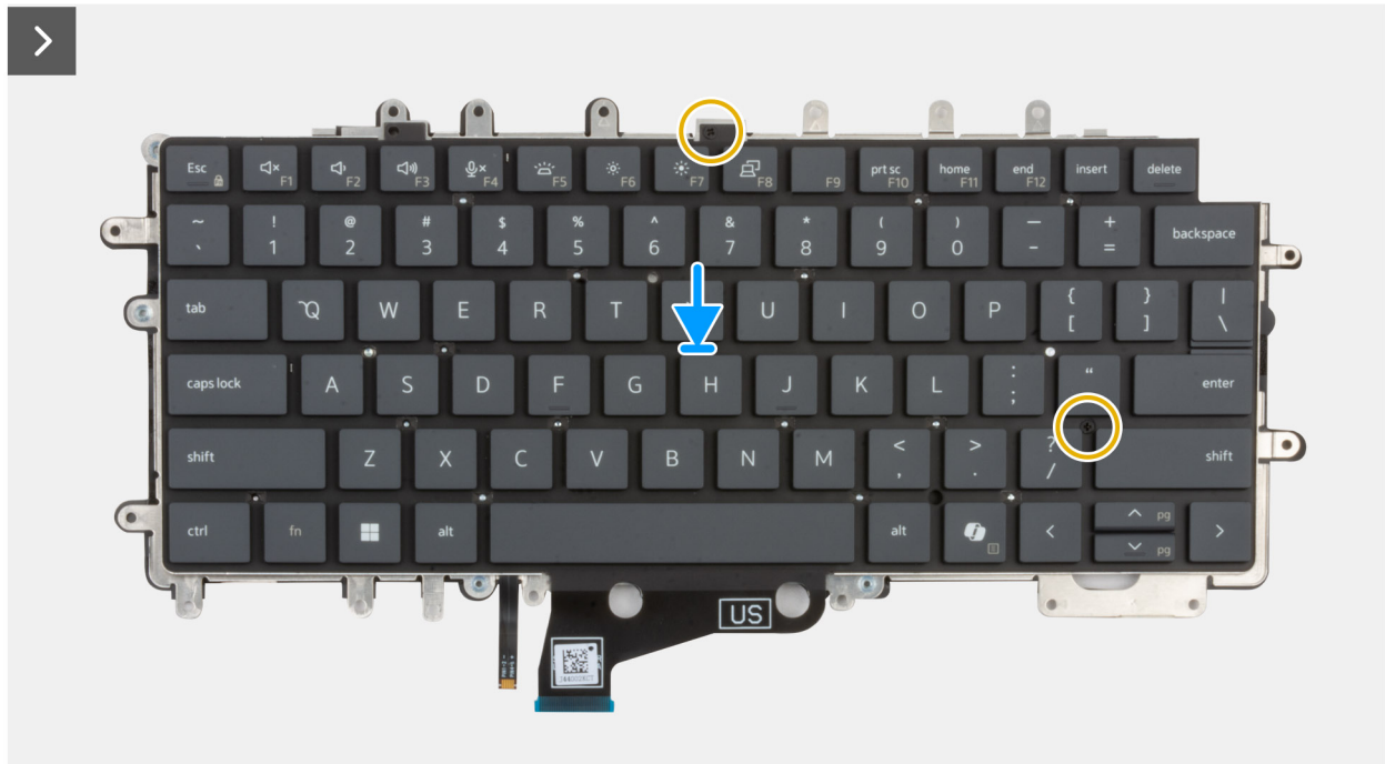
Figure 68. Installing the keyboard
