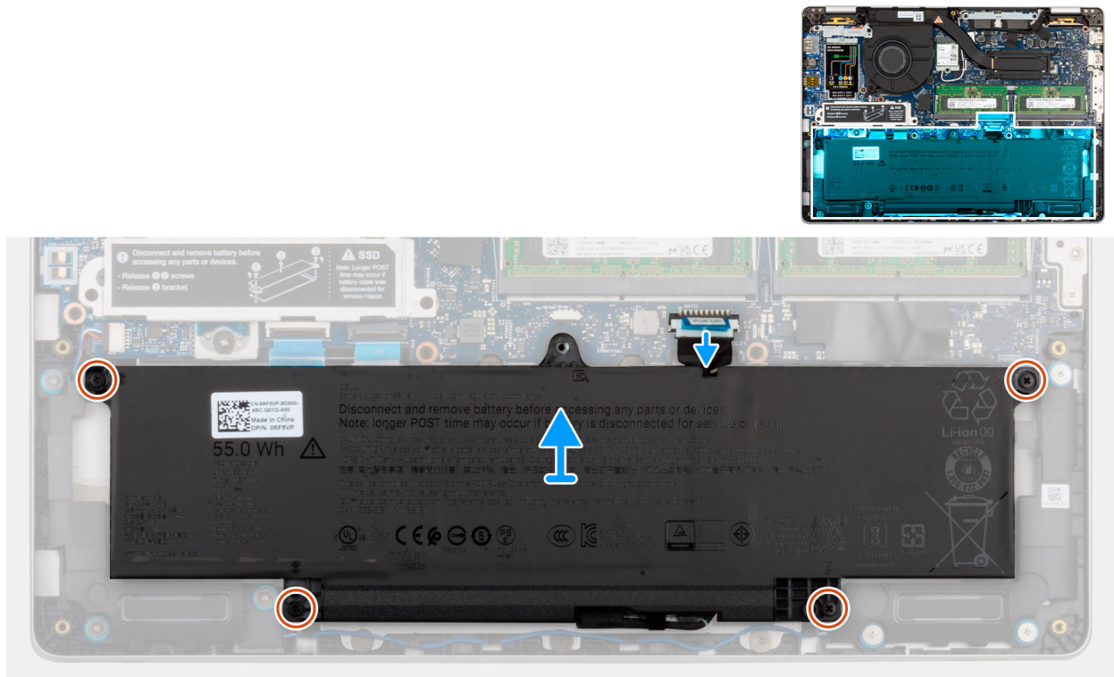
Figure 19. Disconnecting the battery cable
