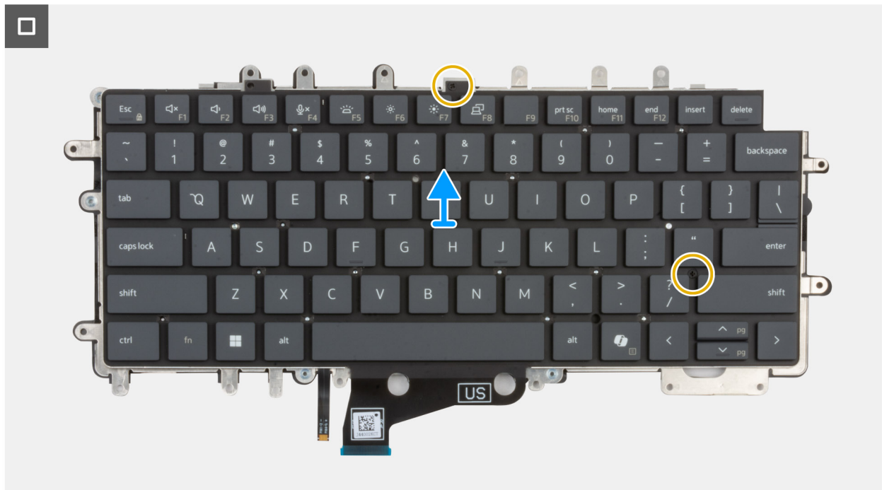
Figure 67. Removing the keyboard
