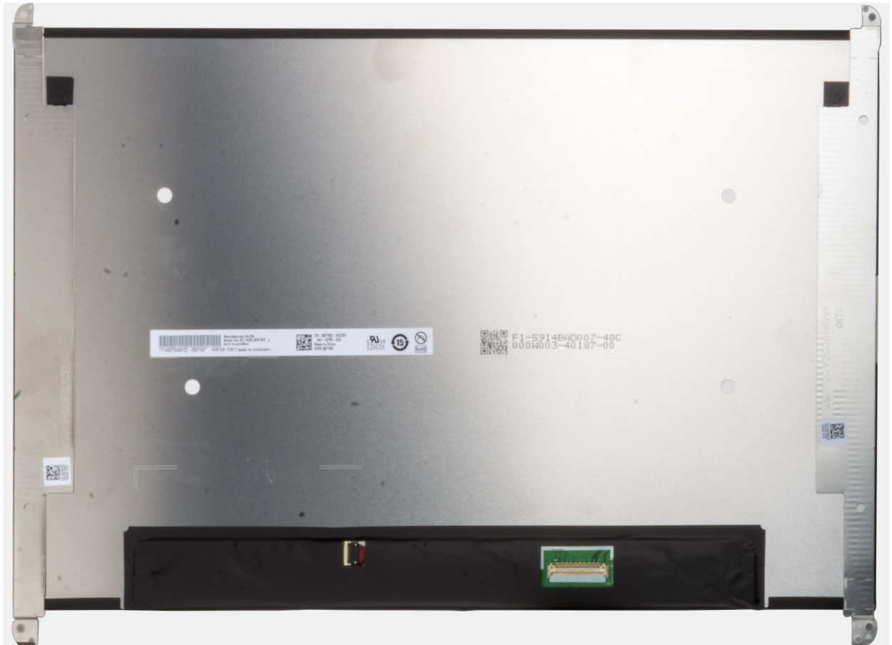
Figure 77. Display panel with brackets
