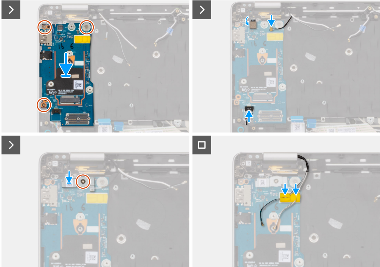
Figure 61. Installing the I/O board
