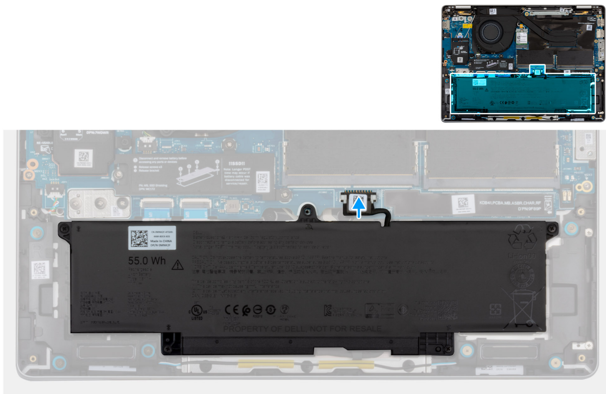
Figure 25. Connecting the battery cable
