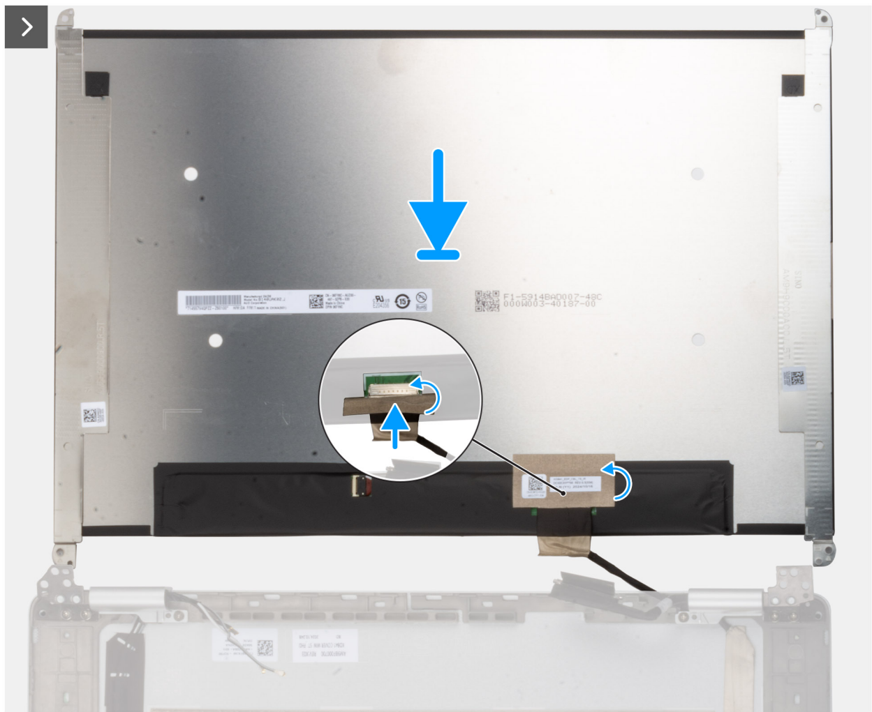
Figure 78. Installing the display panel
