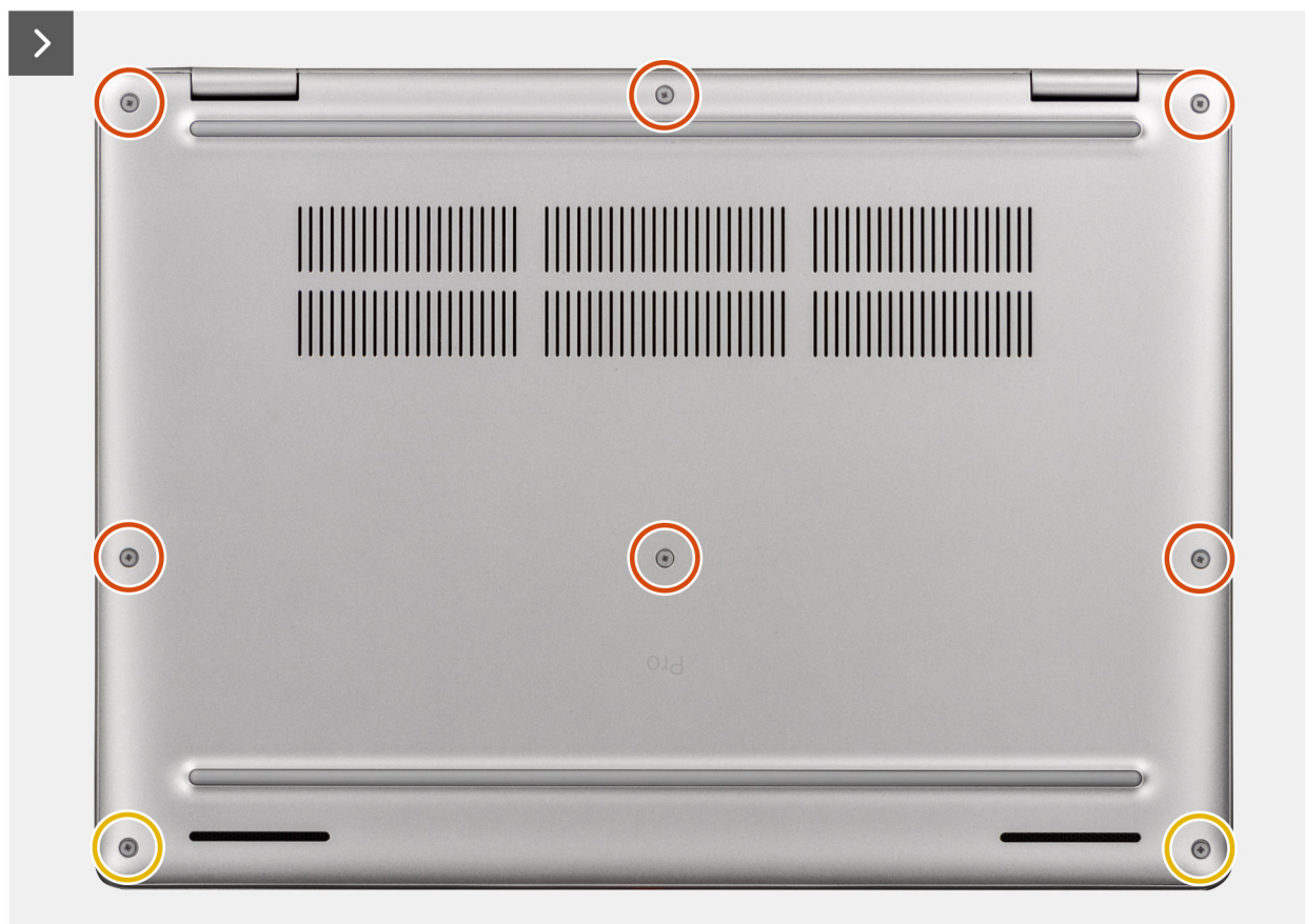
Figure 22. Removing the base cover
