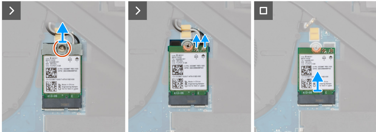
Figure 40. Removing the WLAN card
