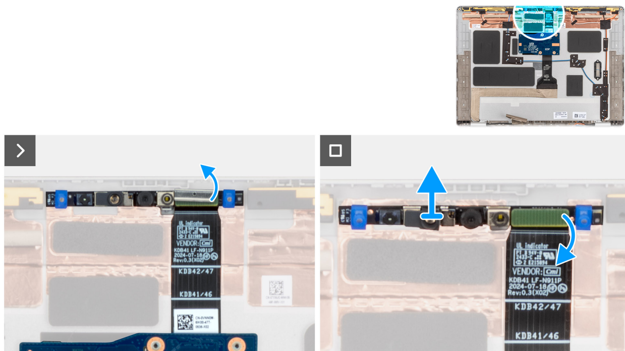
Figure 88. Removing the MIPI camera
