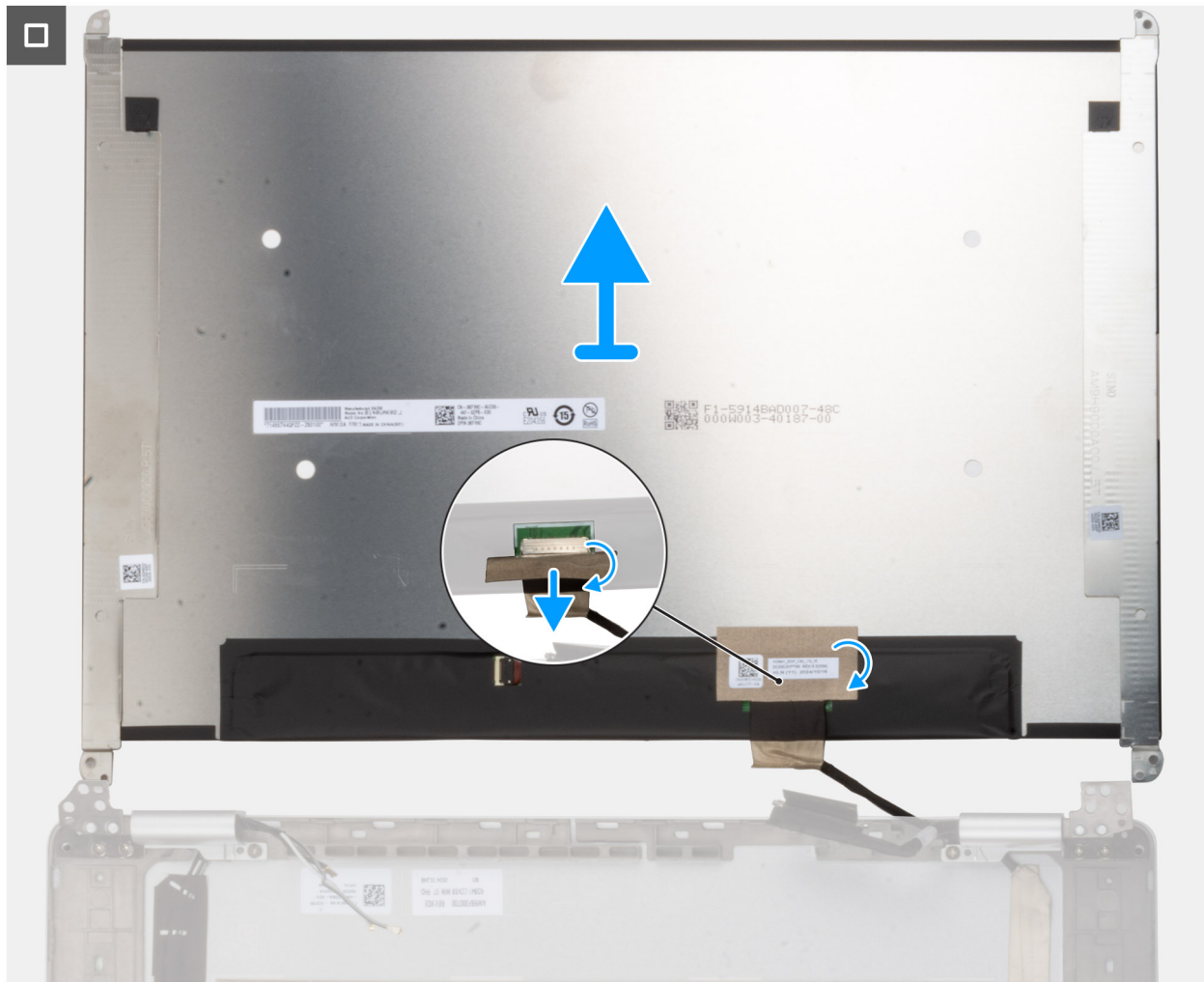
Figure 76. Removing the display panel
