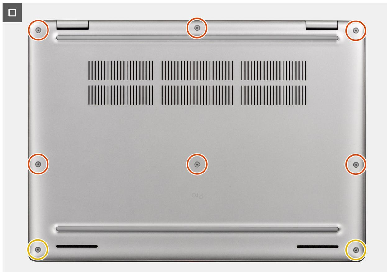
**Figura27. Installing the base cover**
