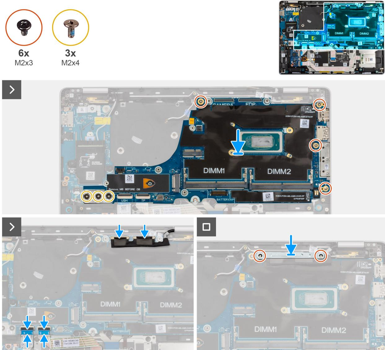
Figura53. Installing the system board
