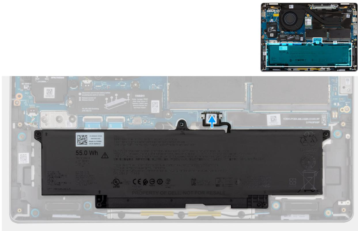
Figura25. Connecting the battery cable
