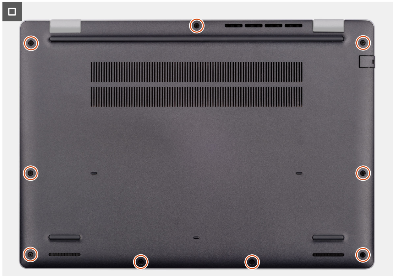
Figure 16. Installing the base cover
