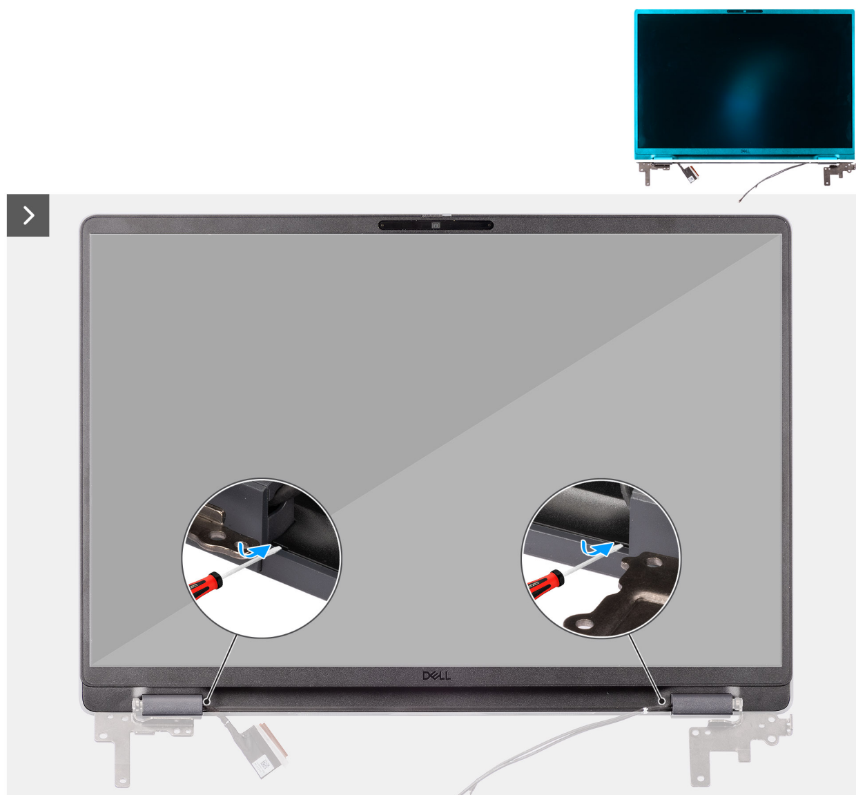
Figure 67. Removing the display bezel
