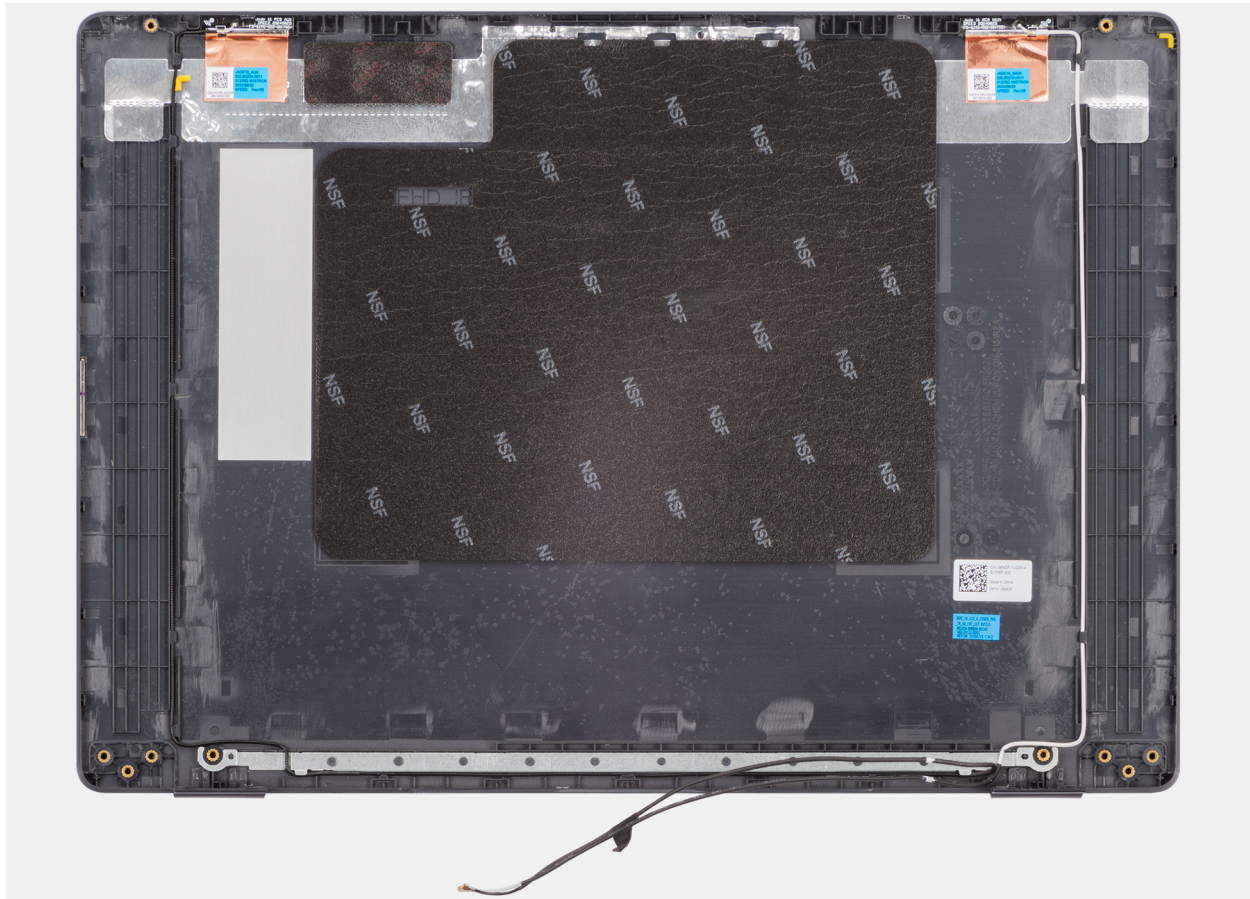
Figure 86. Removing the display back-cover assembly
