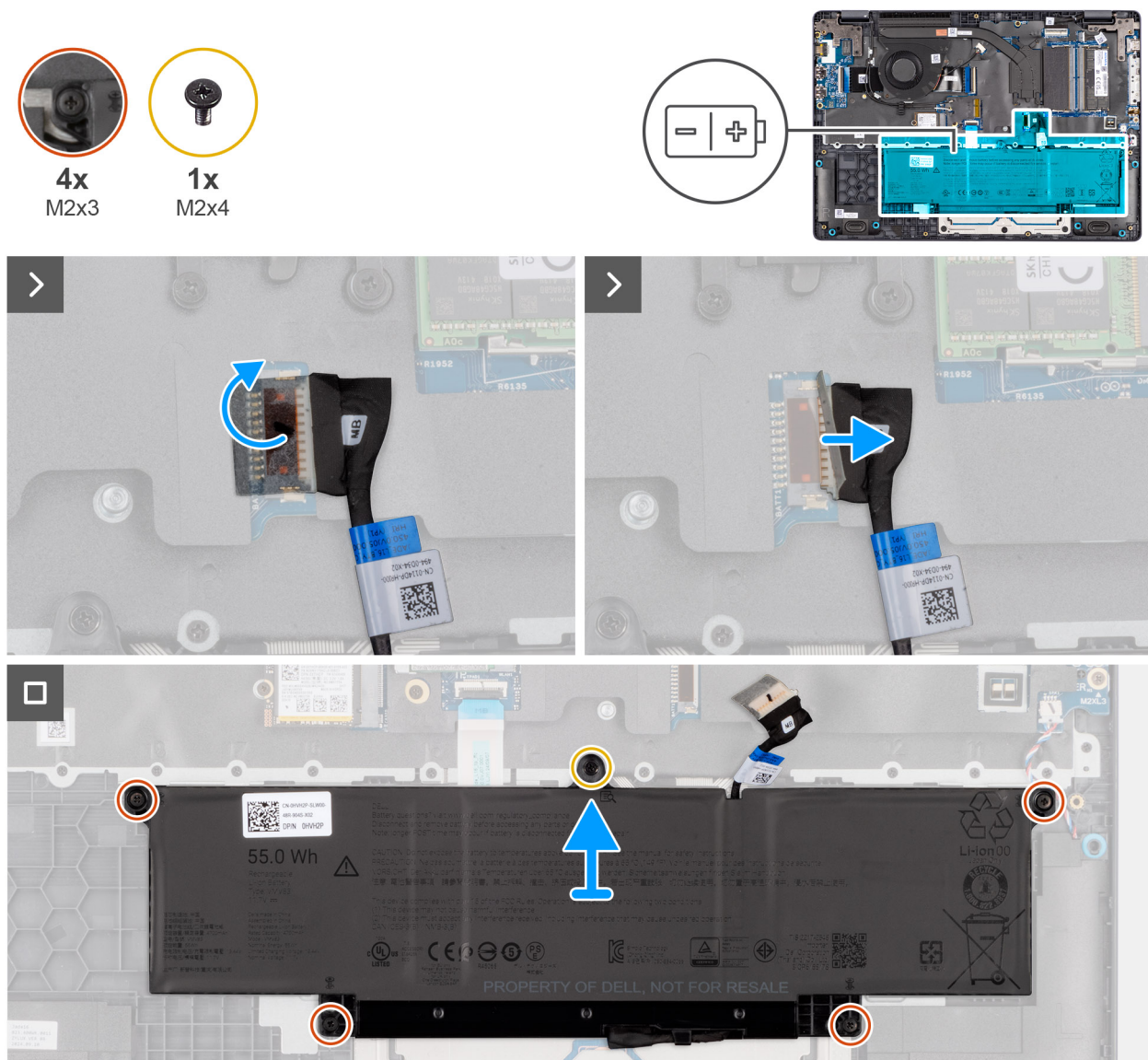
Figure 17. Removing the battery
