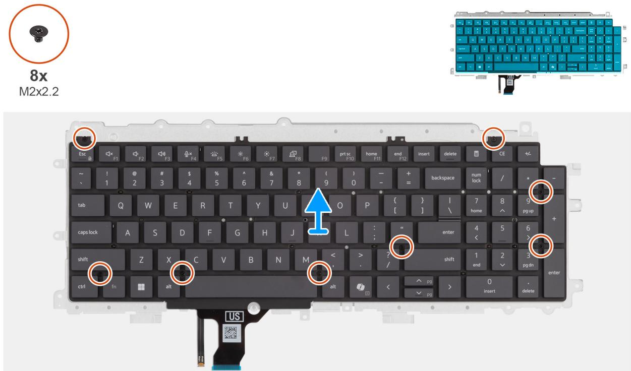
Abbildung 66. Removing the keyboard support plate
