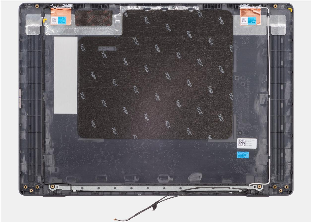
Abbildung 96. Removing the display back-cover assembly
