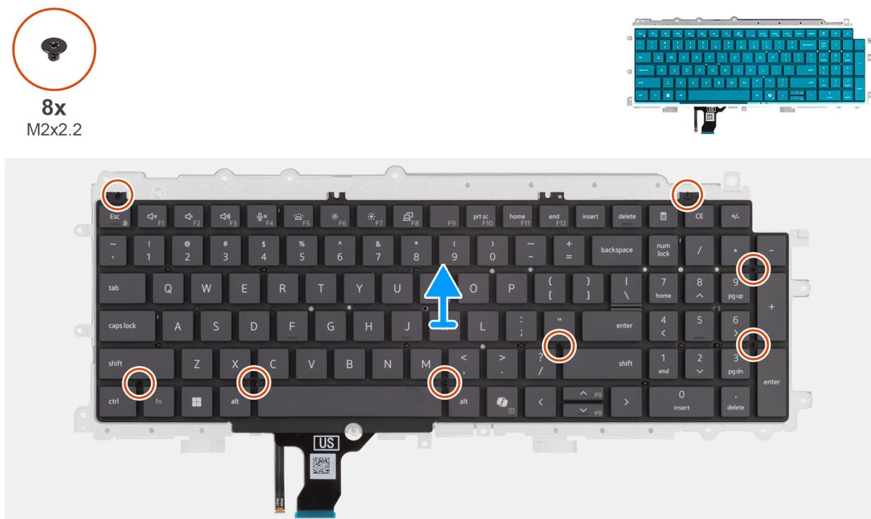
Figure 66. Removing the keyboard support plate
