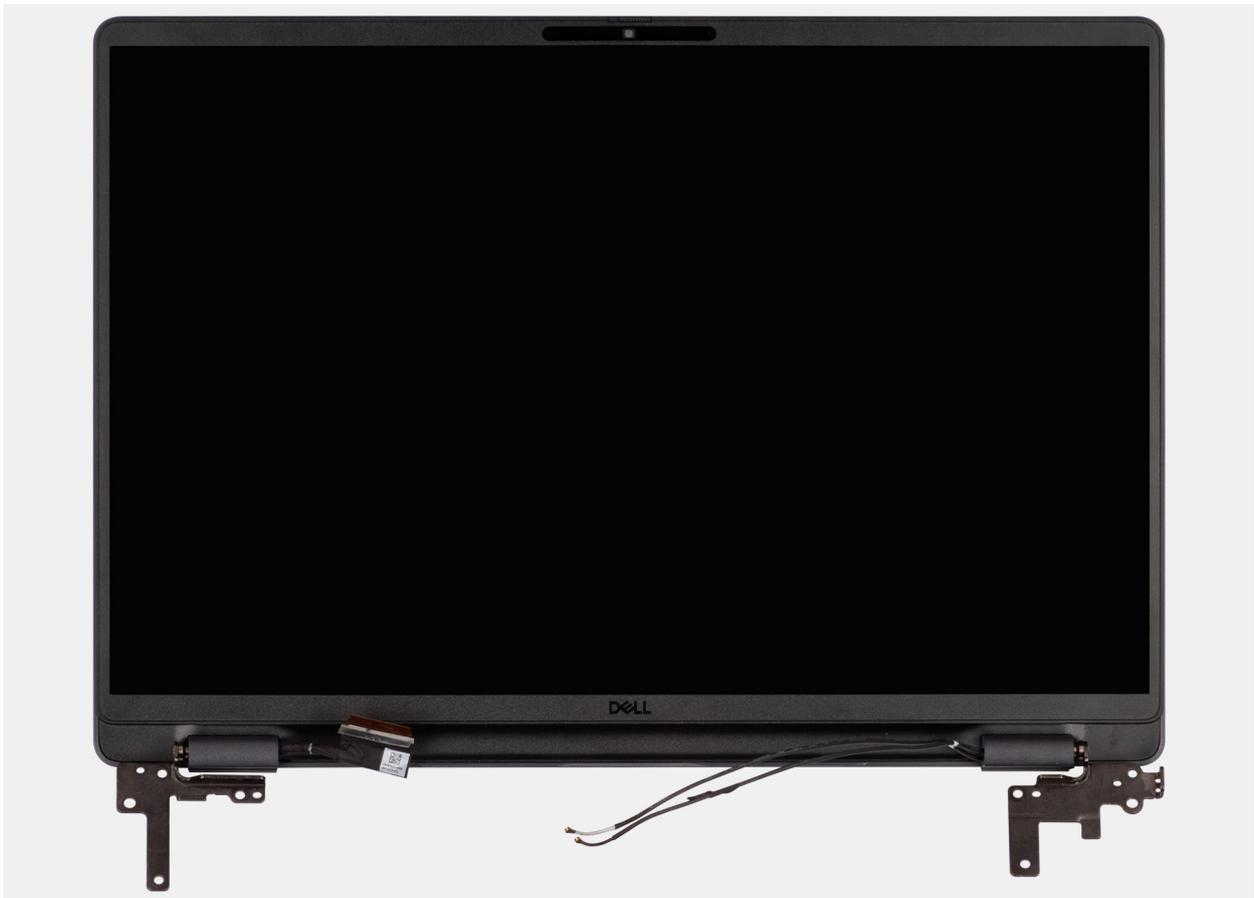
Figure 74. Removing the display assembly
