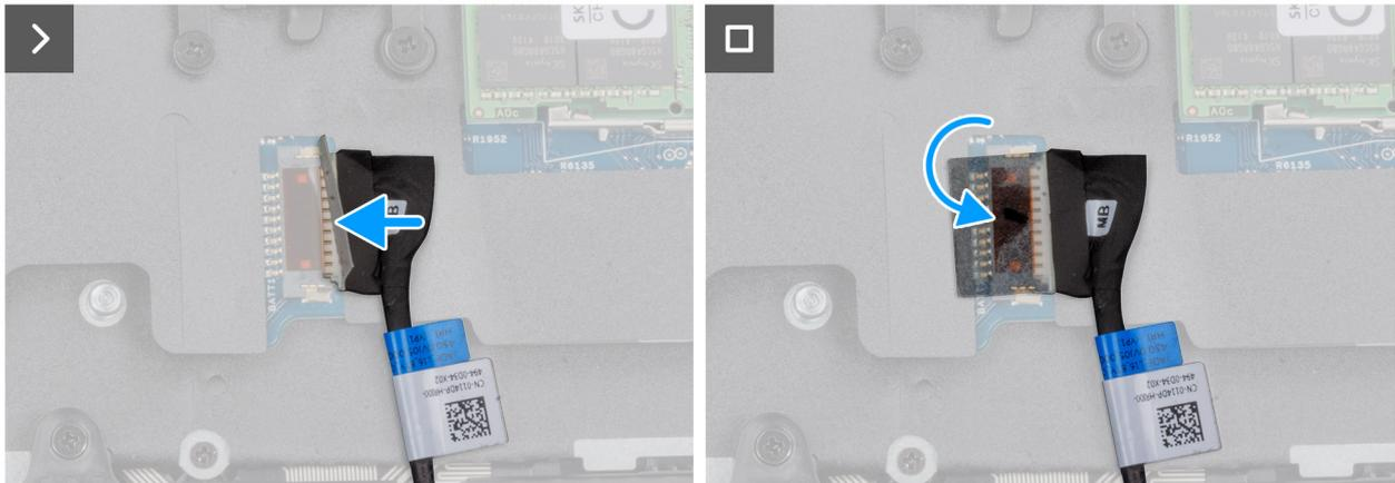
Figure 14. Connecting the battery cable
