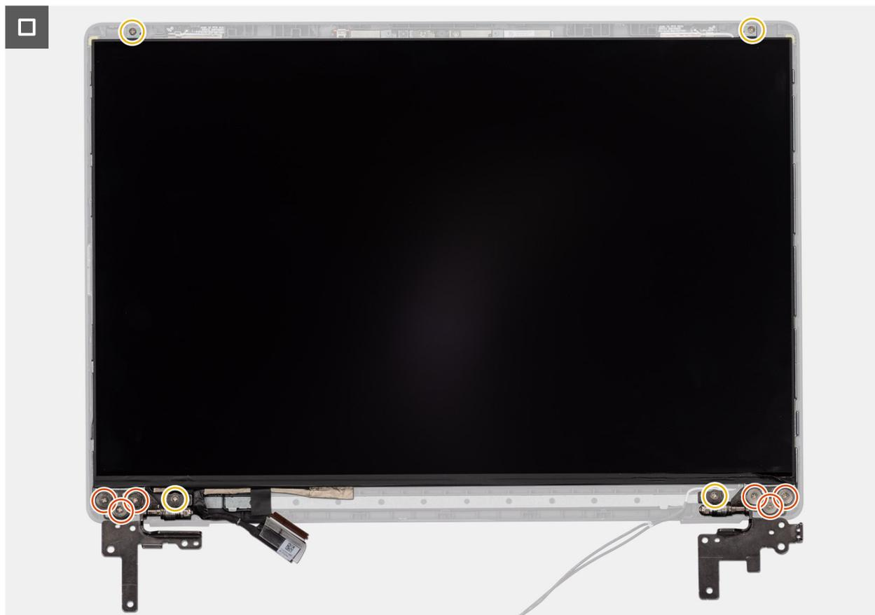
**Figure 91. Installing the display-panel assembly**
