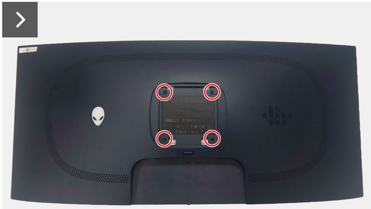
Figure 13. Removing the back cover
