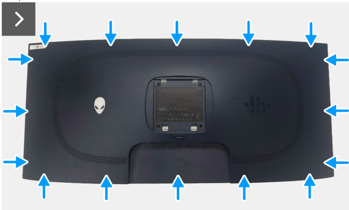
Figure 17. Installing the back cover
