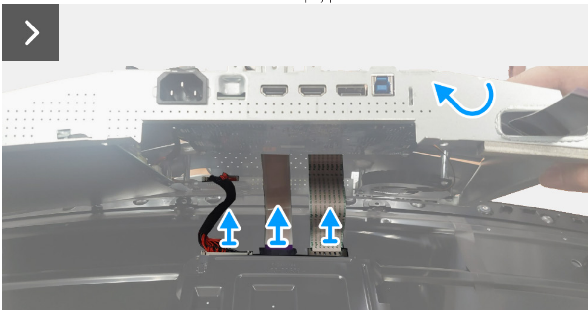
Figure 21. Removing the metal shield
