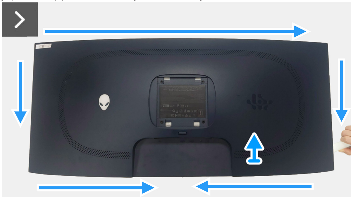
Figure 14. Removing the back cover
