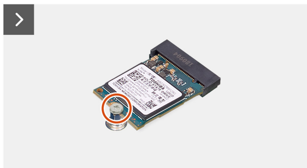
Figure 28. Removing the M.2 2230 solid-state drive in M.2 slot 1
