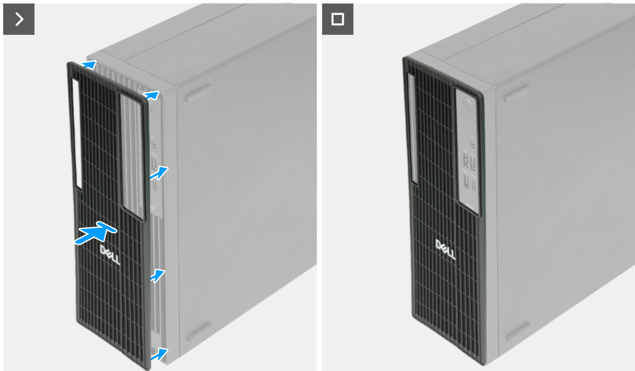
Figure 15. Installation du filtre anti-poussières
