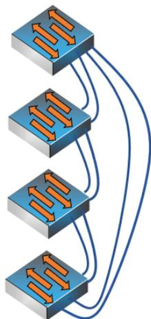
1G models: up to (4) 10G ports per switch can be used for stacking
