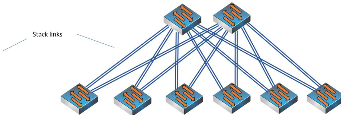
Other models: up to (16) 100G, 25G, or 10G ports per switch can be used for stacking
