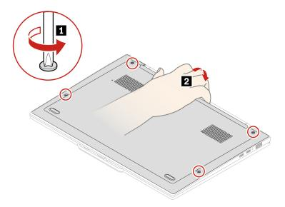
Step 2. Install the base cover assembly in reverse order.
