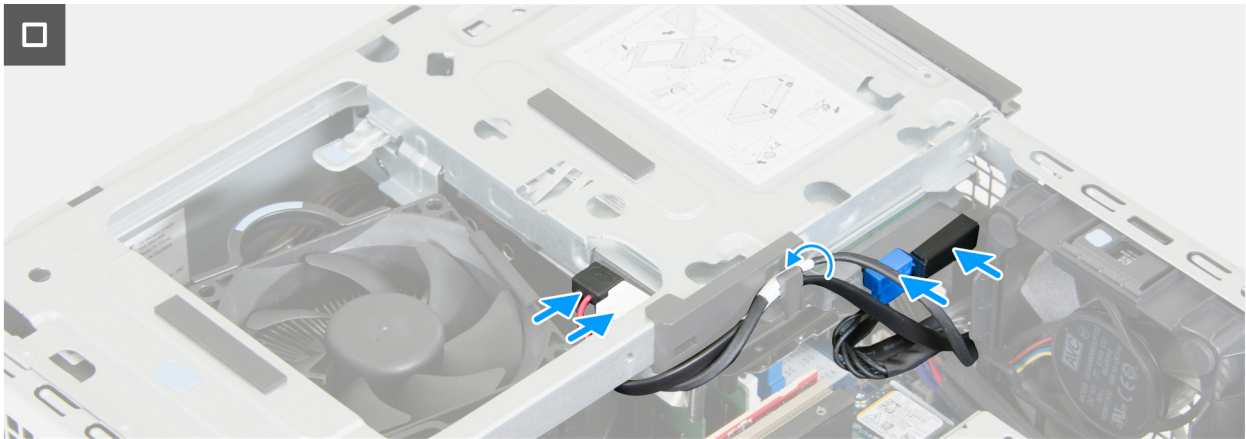
Figure 52. Installing the drive bay
