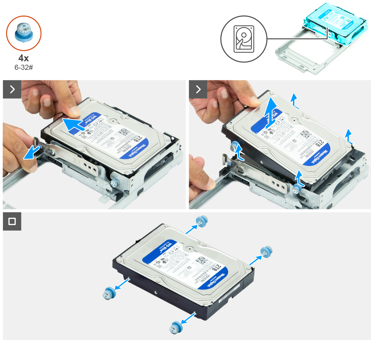
Figure 53. Removing the hard drive
