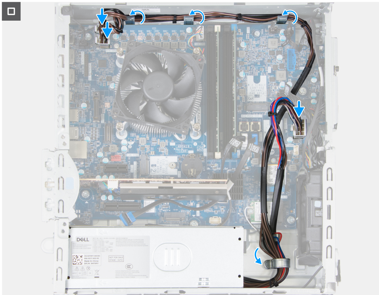
Figure 73. Installing the power-supply unit
