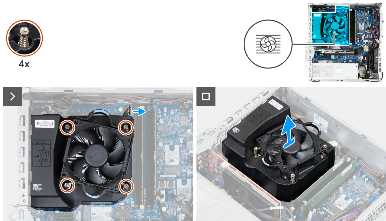
Figure 75. Removing the processor-fan and heat-sink assembly (Dell Pro Slim Plus QBS1250 XE5)
