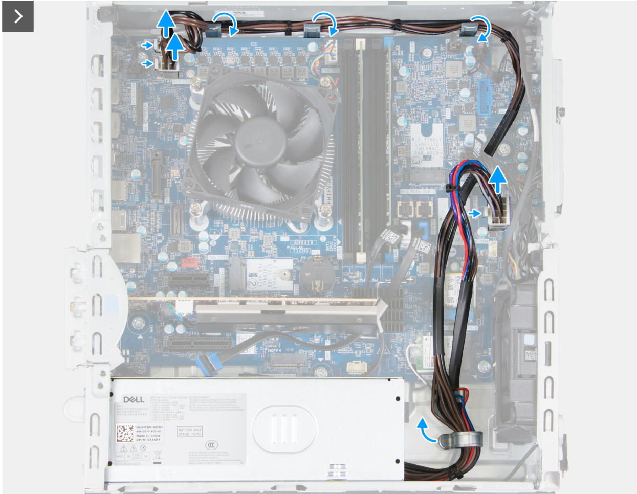
Figure 70. Installing the power-supply unit
