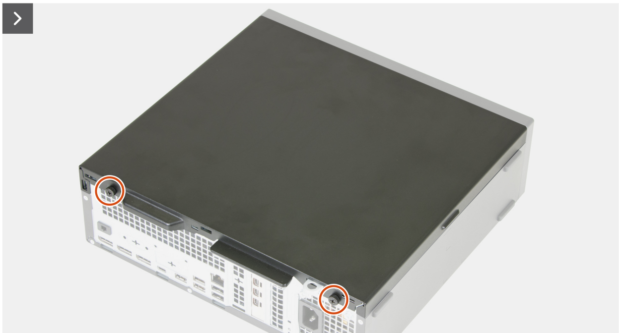
Figure 6. Removing the side cover
