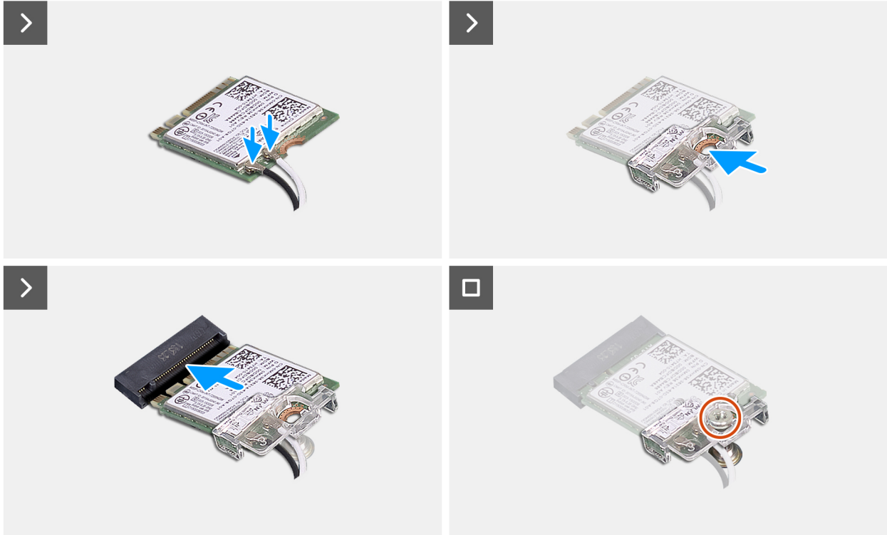
Figure 30. Installing the wireless card
