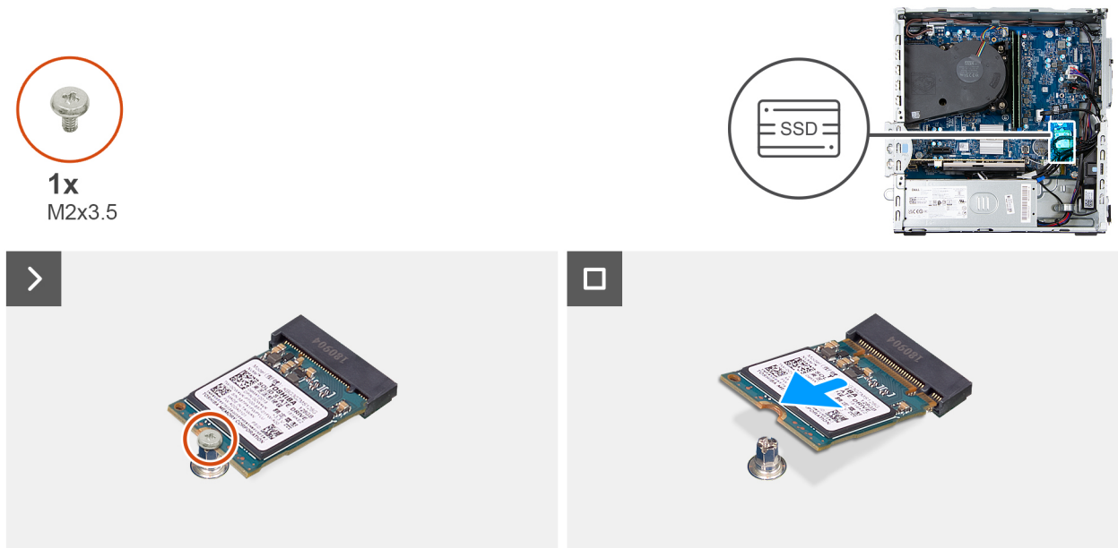
Figure 22. Removing the M.2 2230 solid state drive
