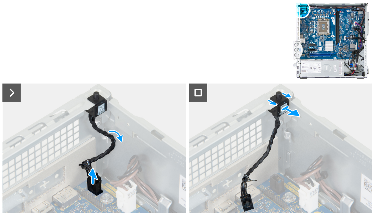
Figure 42. Removing the intrusion switch
