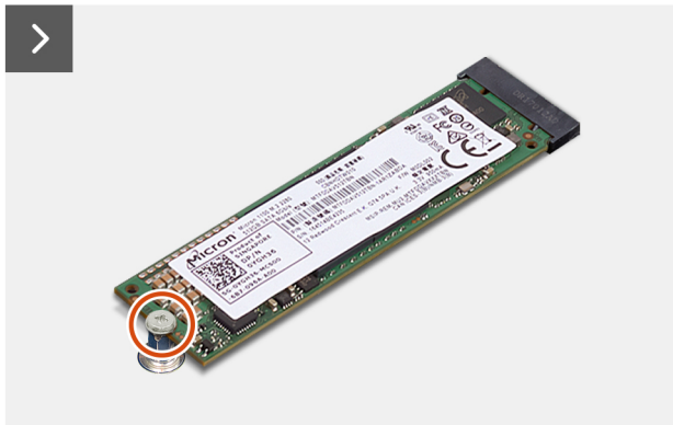
Figure 24. Removing the M.2 2280 solid state drive
