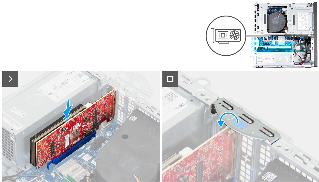
Figure 28. Installing the graphics card
