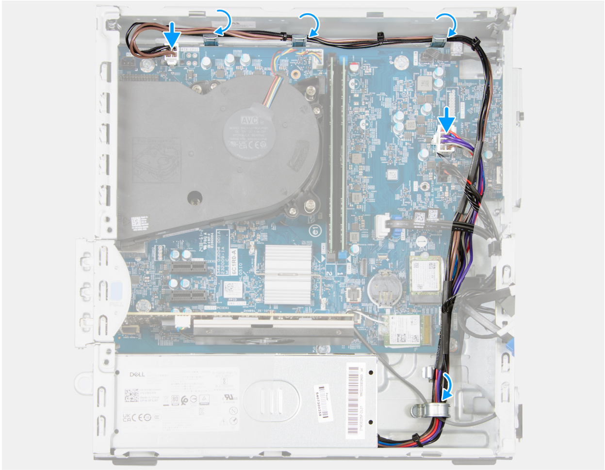
Figure 51. Installing the power-supply unit
