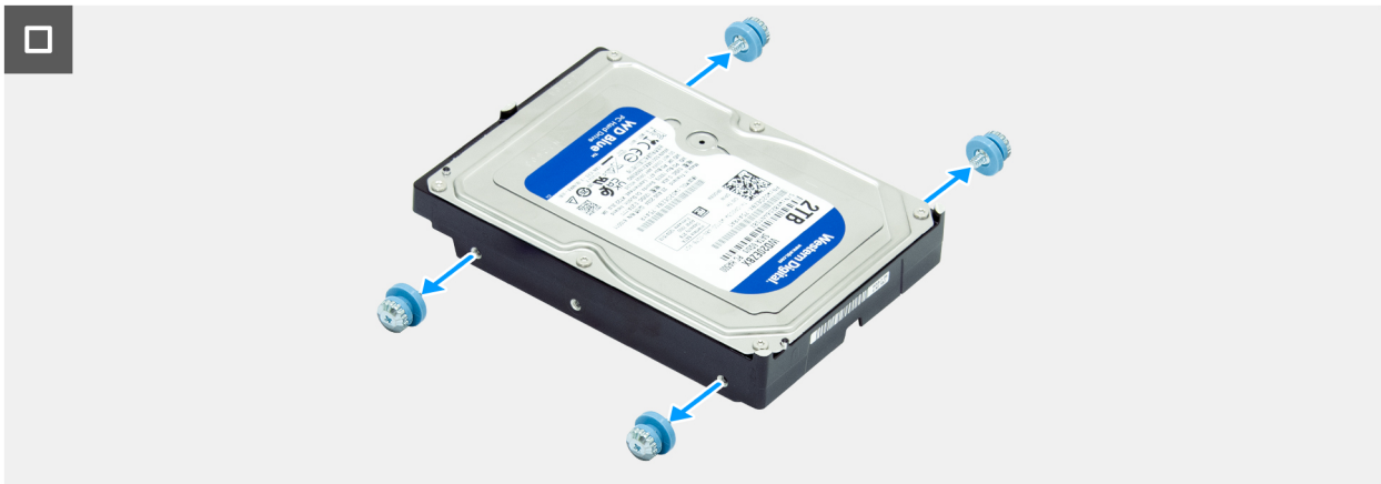
Figure 40. Removing the hard drive
