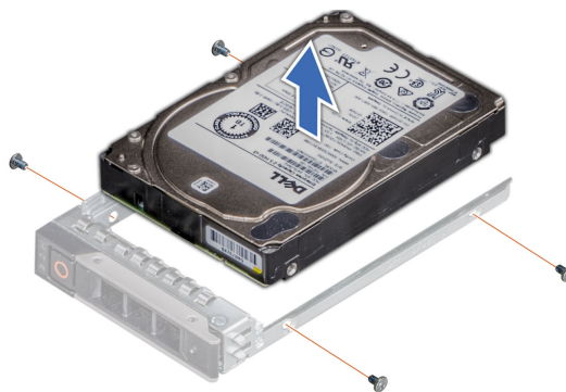
Figure 34. Removing the drive from the drive carrier
