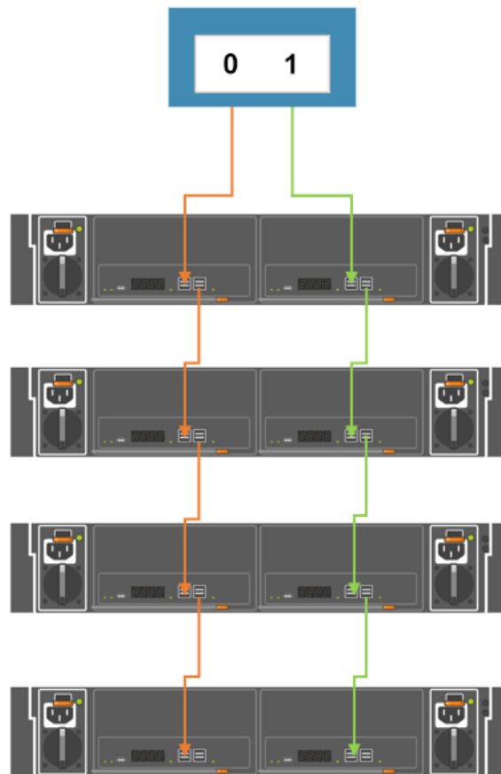
Figure 20. Example of SAS4 redundant-path cabling using a two-port PERC H840
