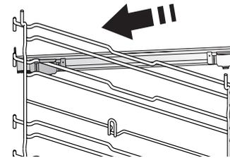
Remove the shelf guides from the oven and remove the protective plastic from the sliding runners.
