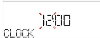
Turn the **adjustment knob** to set the correct hour and press **✓**: The two digits for the minutes will flash on the display. Turn the **adjustment knob** to set the minutes and press **✓** to confirm.
