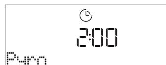
Turn the adjustment knob to select the desired cycle, then press to confirm. Once a cycle has been selected, if desired, turn the adjustment knob to set end time (start delay), then press to confirm. The display will prompt you to do all actions needed to obtain the best cleaning results: Follow the indications and then press when done. Once you have done all steps, when required press to activate the cleaning cycle.
