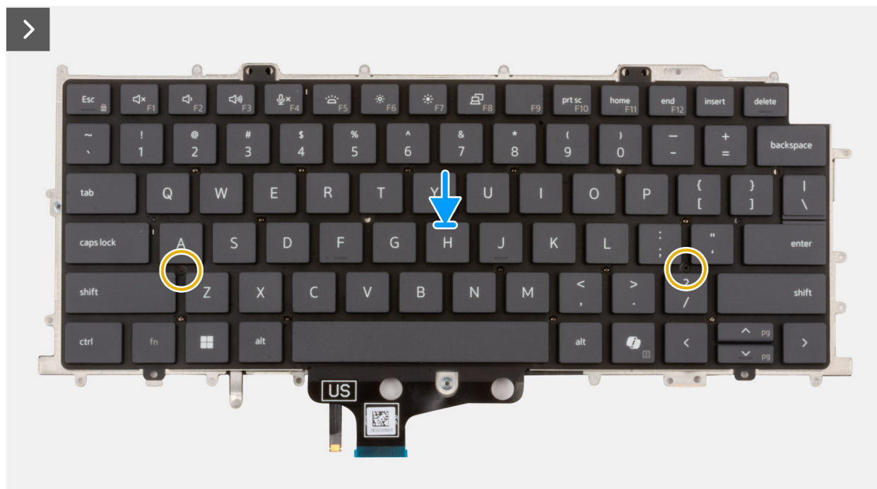
Figure 100. Installation du clavier
