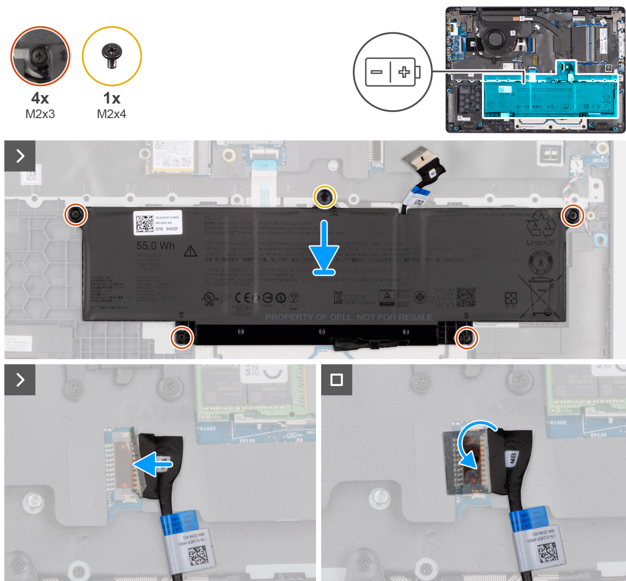
Figure 18. Installing the battery
