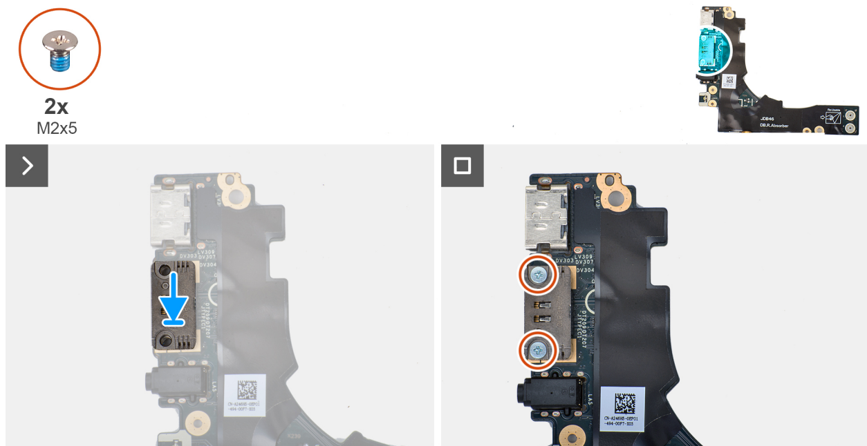
Figur 55. Removing the right USB Type-C module
