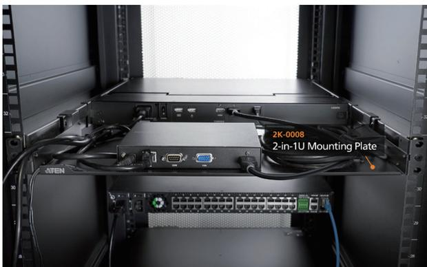
The 2-in-1U Mounting Plate allows you to install an LCD KVM console with KVM over IP console station / extender on the same unit of space as shown above. (This image shows an installation scenario with KA8278 and 2K-0008 combined.)
