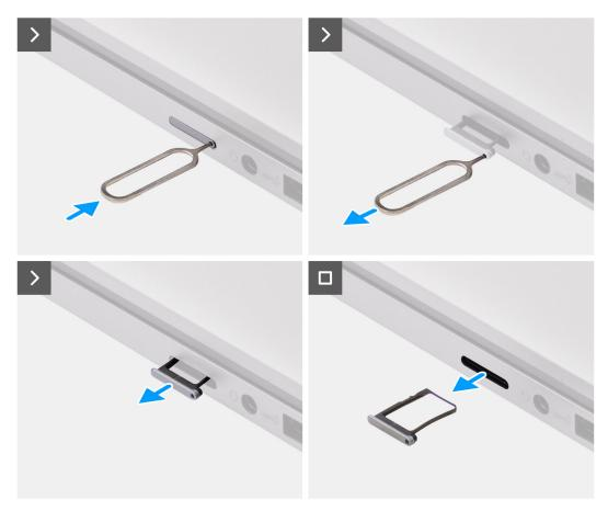
Figure 3. Removing the SIM-card tray from the computer
