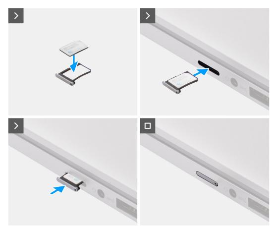
Figure 4. Installing the SIM card into the computer
