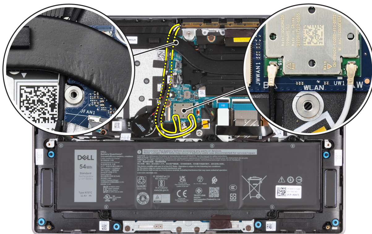
Figure 62. Installing WLAN-antenna cables
