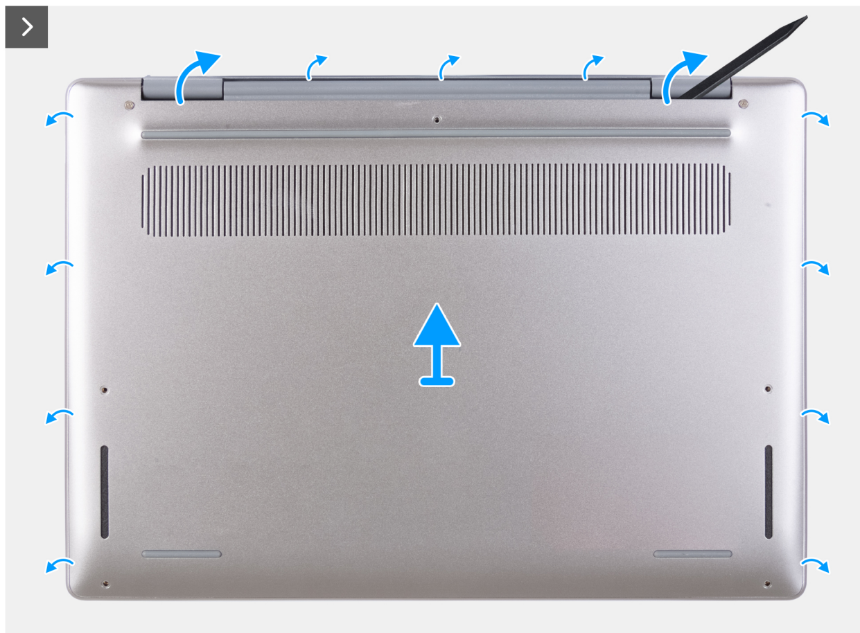
Figure 16. Removing the base cover
