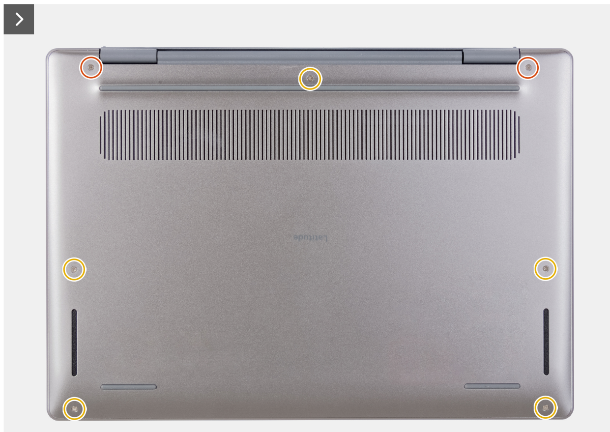
Figure 15. Removing the base cover
