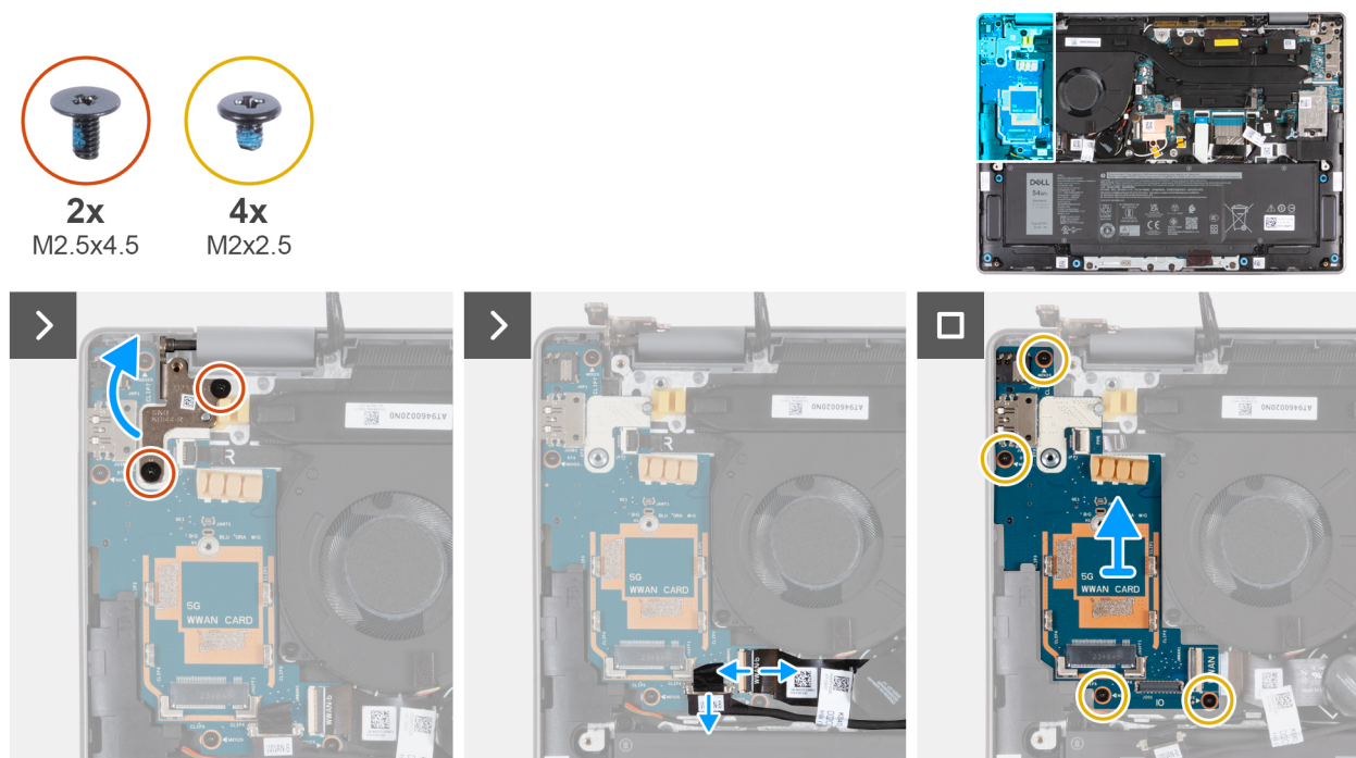
Figure 84. Removing the I/O board (for computers shipped with WWAN support)
