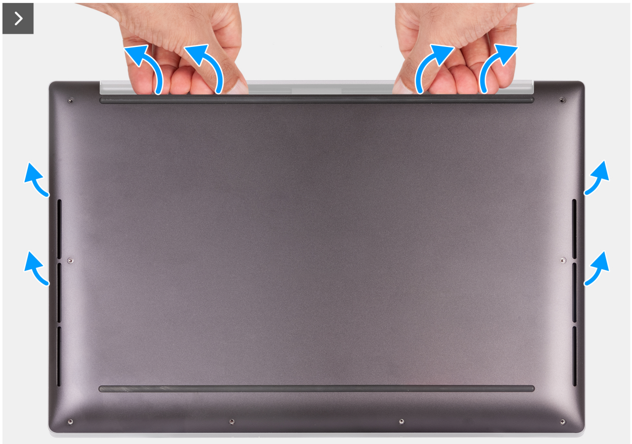
Figure 2. Using both thumbs to pry the base cover
