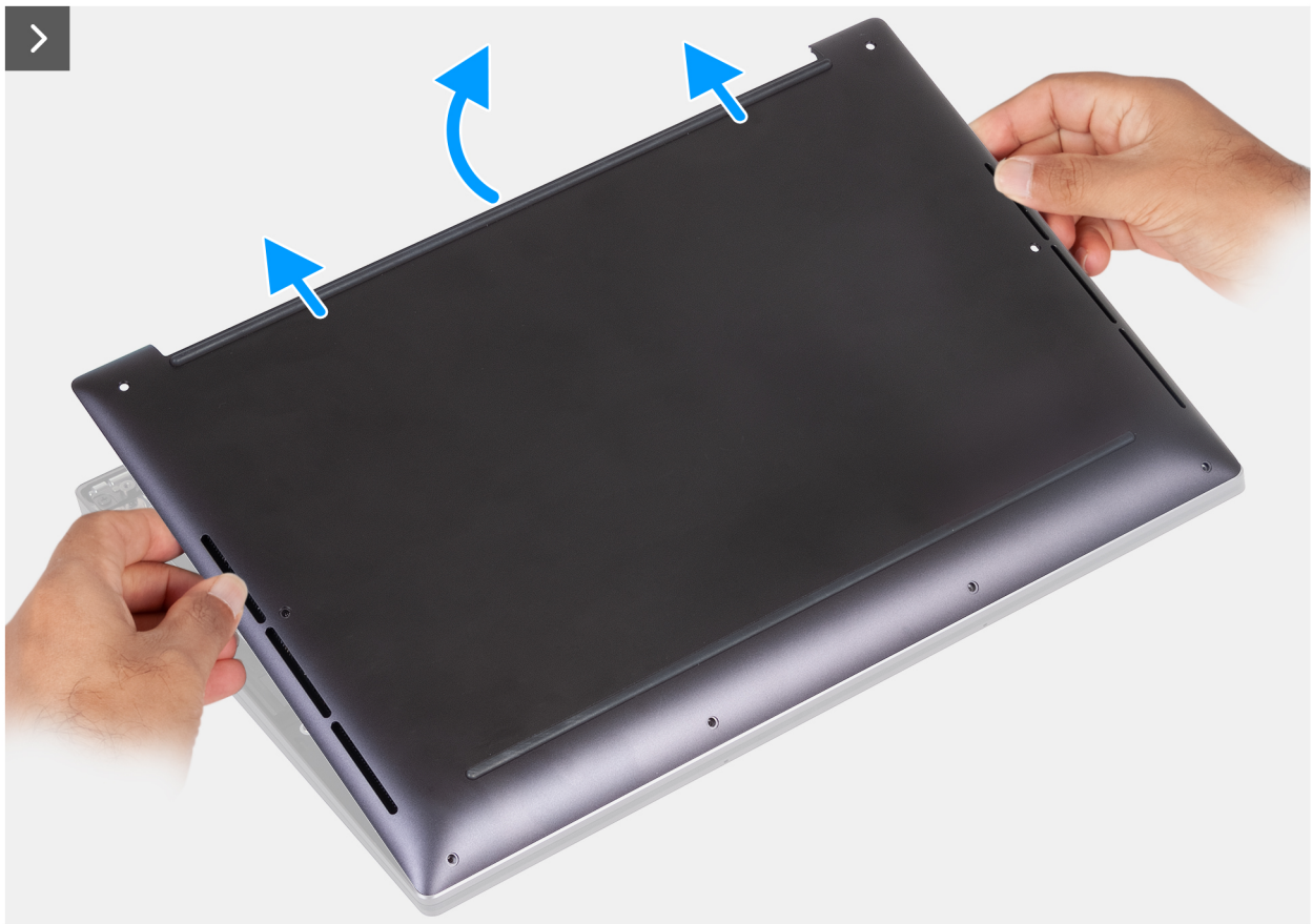
Figure 3. Lifting the base cover off the palm-rest assembly
