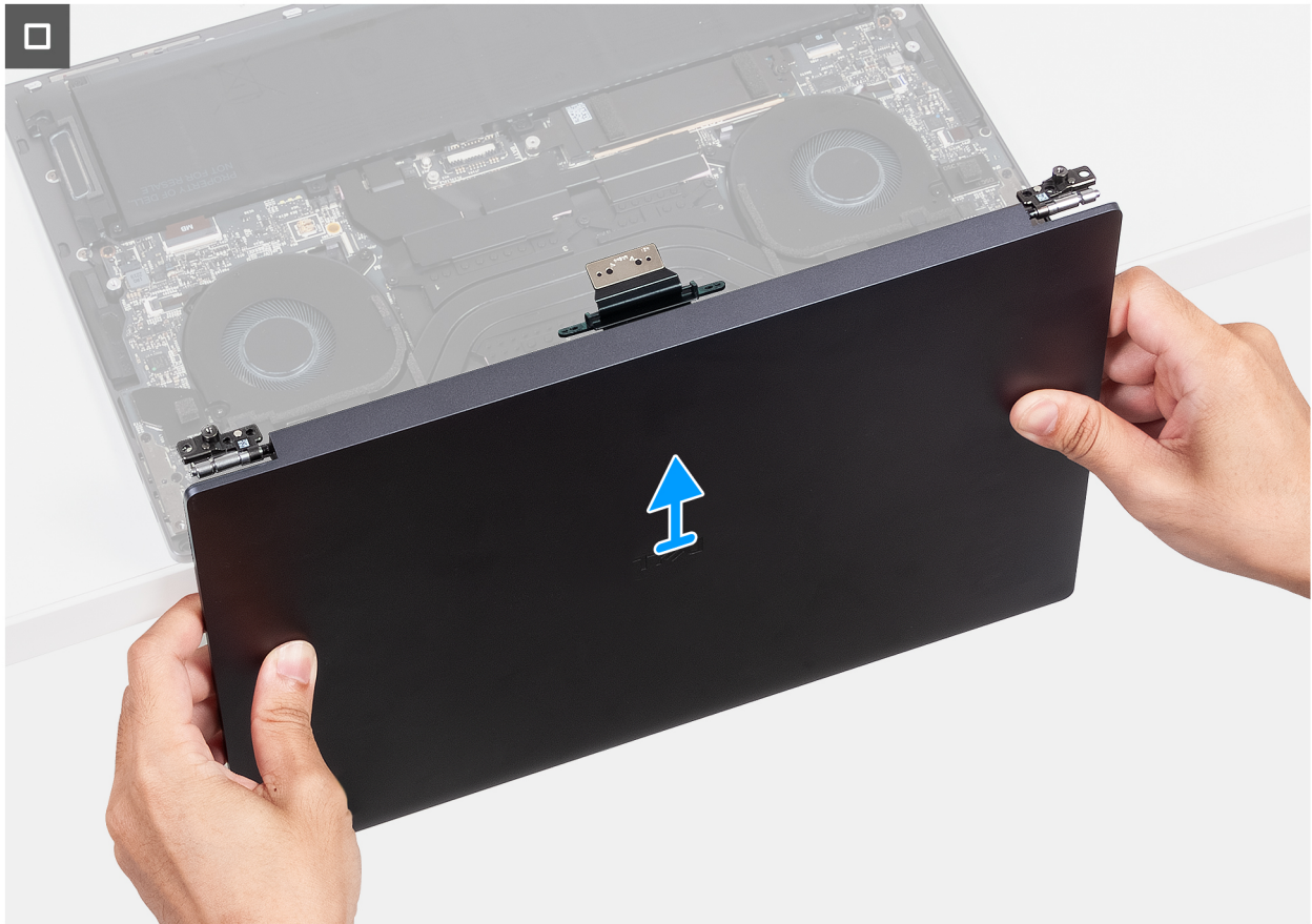
Figure 20. Removing the display assembly
