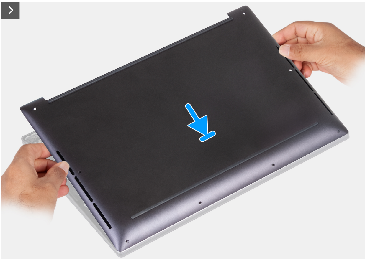
Figure 6. Placing the base cover into slots on the palm-rest assembly
