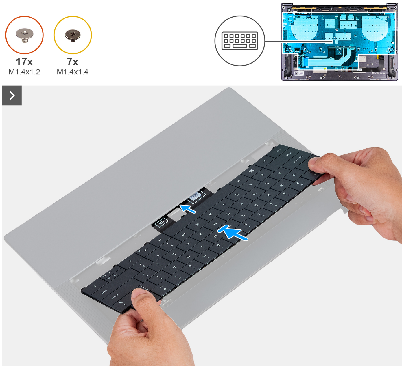
Figure 34. Installing the keyboard
