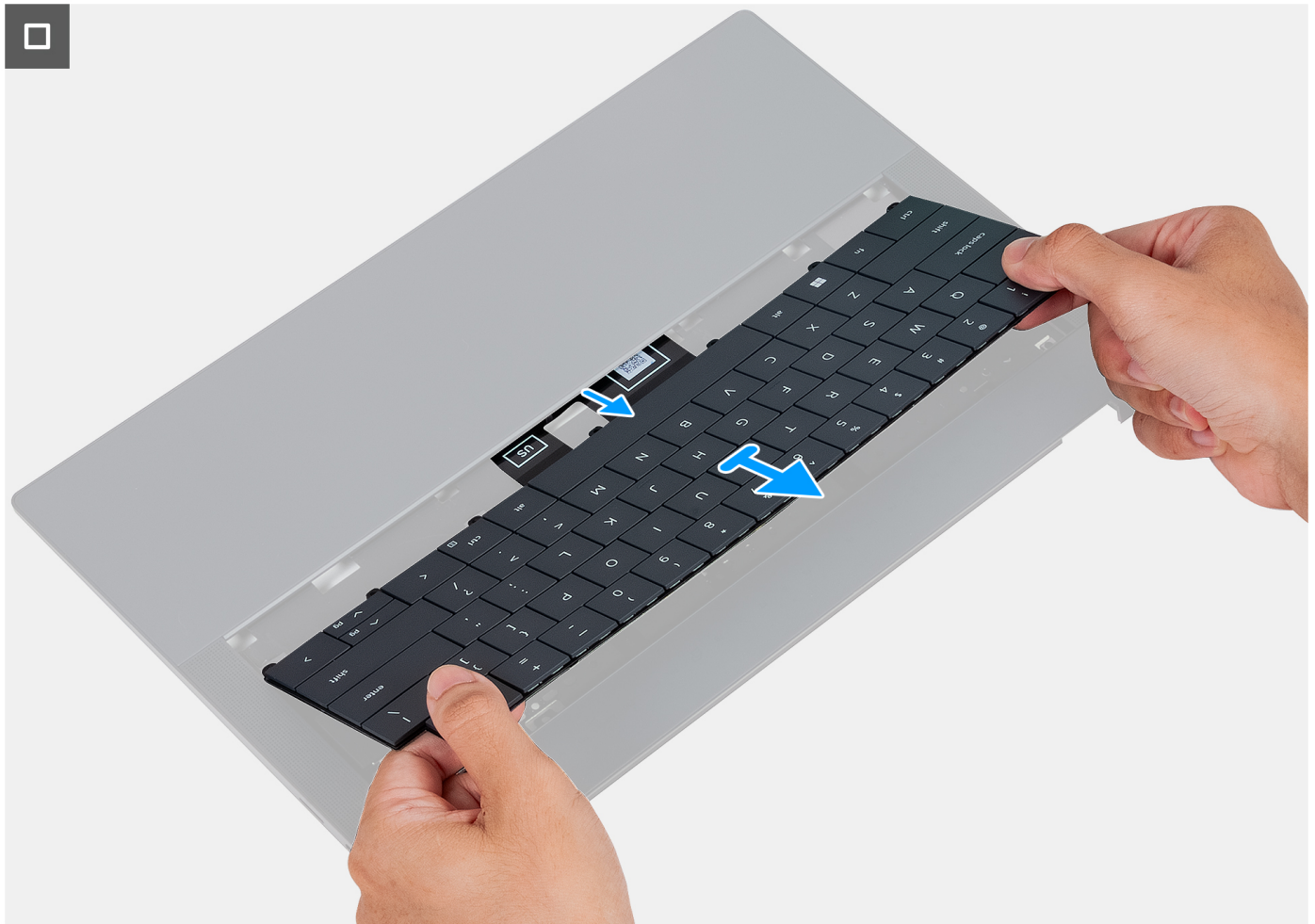
Figure 33. Removing the keyboard
