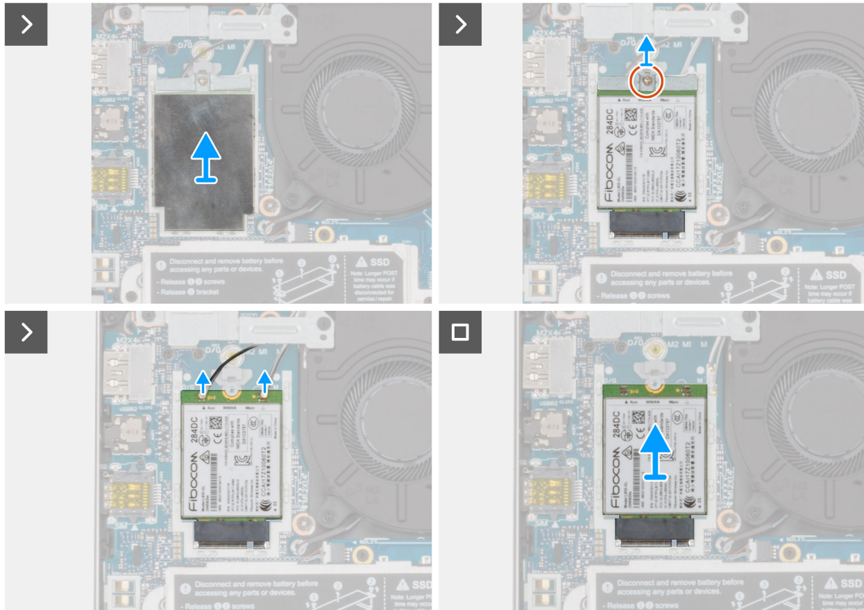
Figure 30. Removing the 5G WWAN card
