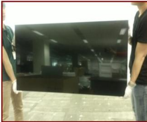
Move LCM in vertical status to prevent LCM bent.
